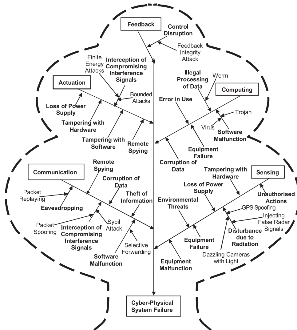
Fig. 2. A tree diagram of attacks and threats on cyber-physical systems.
