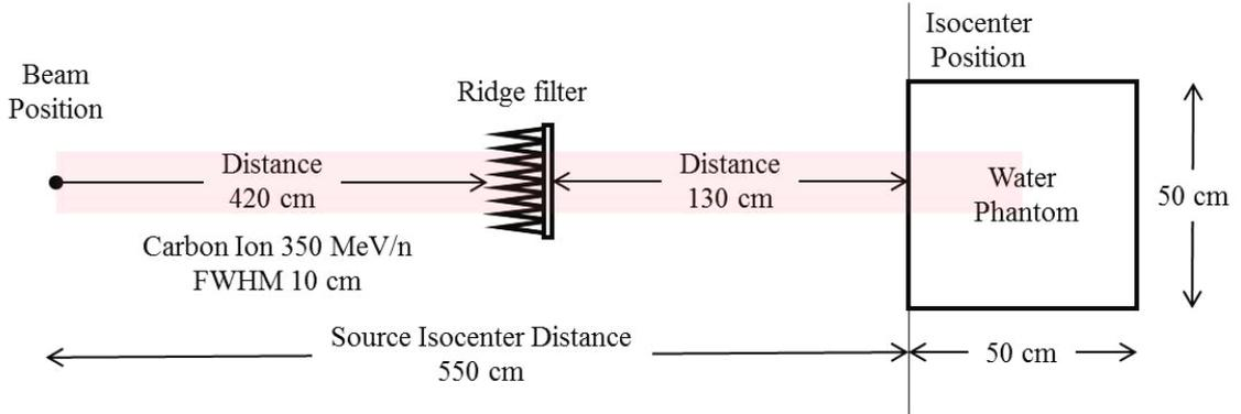
Fig. 2. (Color online) Schematic layout of the broad-beam delivery system used in the Monte Carlo simulation.
