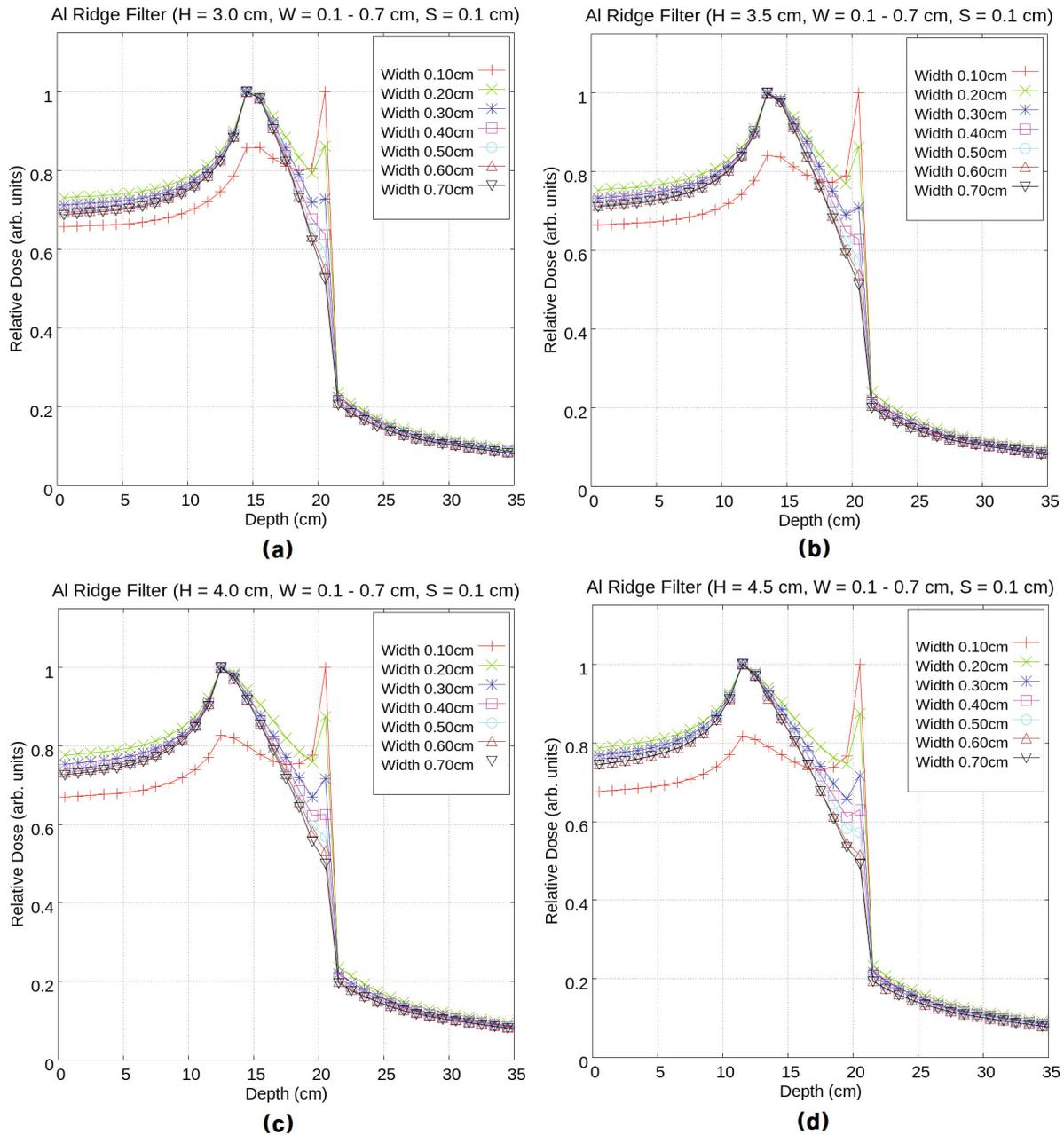
Fig. 6. (Color online) The physical dose distribution in a carbon-ion beam of 350 MeV/n was determined using the FLUKA 2011 code. The heights of the ridge filters are (a) 3.0 cm, (b) 3.5 cm, (c) 4.0 cm and (d) 4.5 cm. The width of the ridge filter was varied from 0.05 cm to 0.7 cm in intervals of 0.05 cm.
