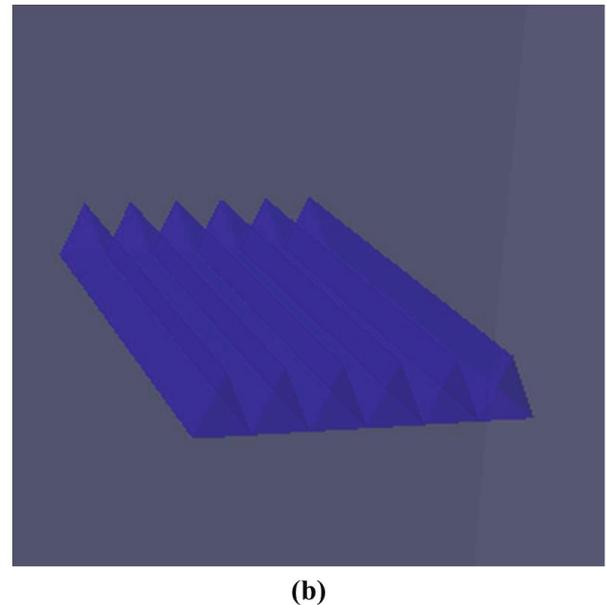
Fig. 4. (Color online) (a) Geometry layout and (b) the ridge filter in GEANT4.
