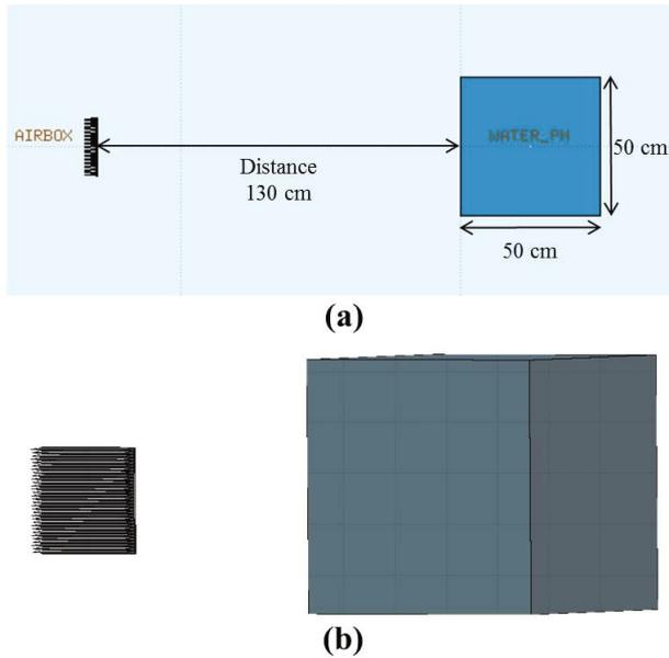
Fig. 3. (Color online) Geometry of the (a) 2D view and (b) 3D view in FLUKA.
