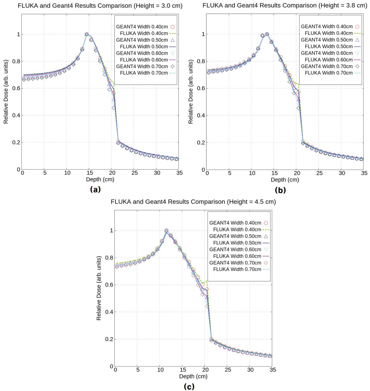
Fig. 7. (Color online) Data calculated by using the FLUKA and the GEANT4 codes are compared to the physical dose calculated. The heights of the ridge filter were (a) 3.0cm, (b) 3.8cm and (c) 4.5 cm.
