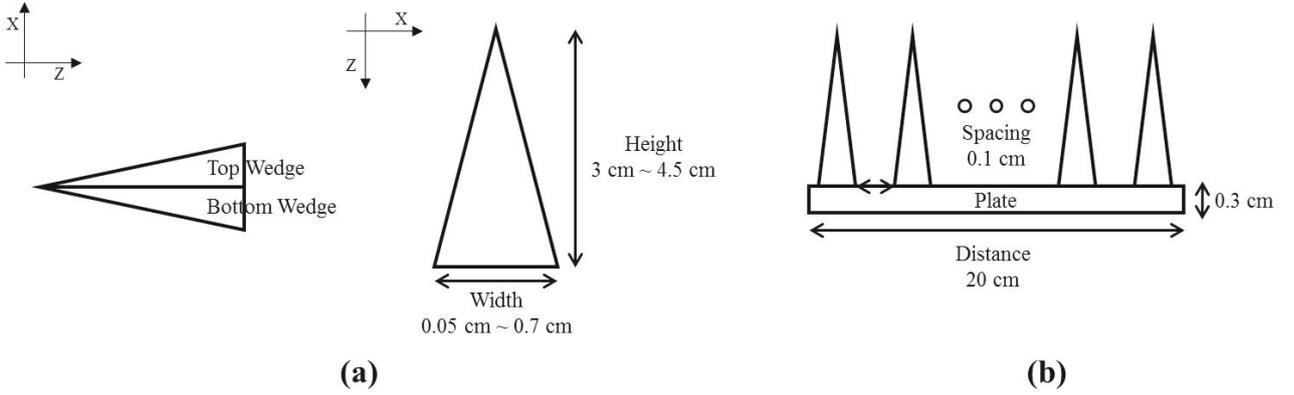
Fig. 1. Schematic of the groove design of the ridge filter.
