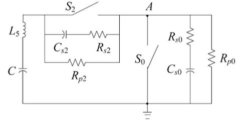
Fig. 6. Equivalent circuit of the control valve and test valve.
