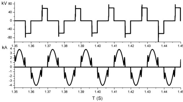
Fig. 5. Current and voltage waveforms of the test valve for double injection test of thyristor controlled reactor (TCR) valves.
