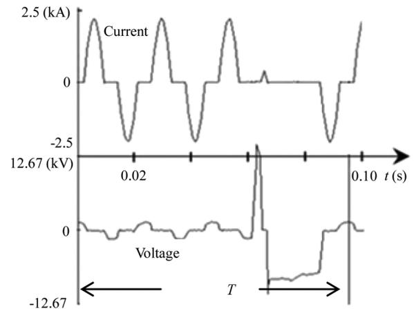
Fig. 12. Waveforms of the operational test on Wanxian TCR valve.
