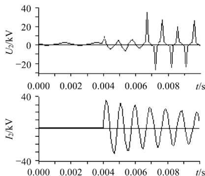
Fig. 7. Simulated voltage and current waveforms without overvoltage protection for the transformer.
