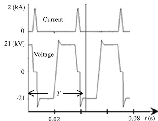
Fig. 13. Test waveforms of the operational test on the Yifeng TCSC valve.
