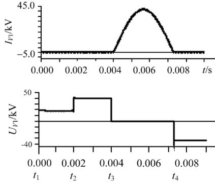
Fig. 4. Waveforms under the overcurrent mode.
