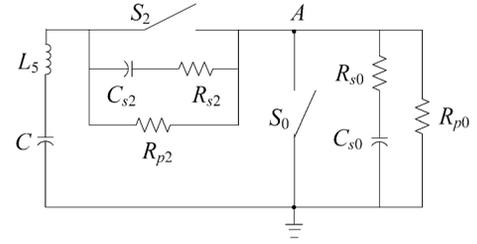
Fig. 6. Equivalent circuit of the control valve and test valve.
