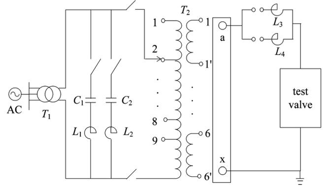
Fig. 2. Schematic diagram of the temperature-rise mode.
