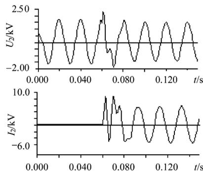
Fig. 9. Simulated voltage and current waveforms of protection valve with BOD.
