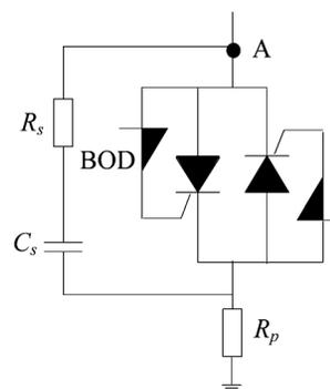
Fig. 8. Schematic diagram of the protection strategy.
