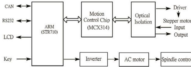
Figure 2. The block diagram of the overall structure of hardware
