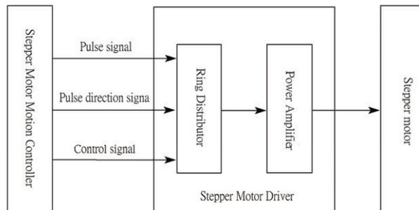
Figure 4. Open-loop control system structure of stepper motor
