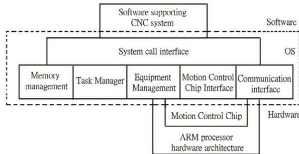
Figure 1. The overall structure model of CNC system
