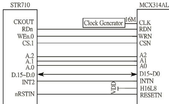
Figure 3. The connection diagram of STR710 and MCX314AL
