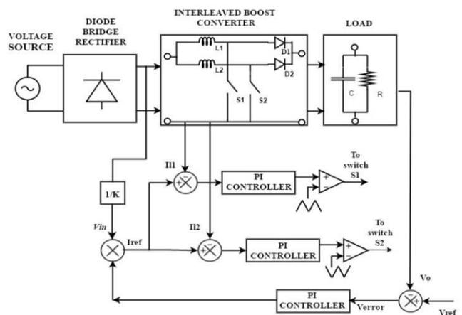
**Figure-4.** Block diagram of analog control of Interleaved Boost Converter.
