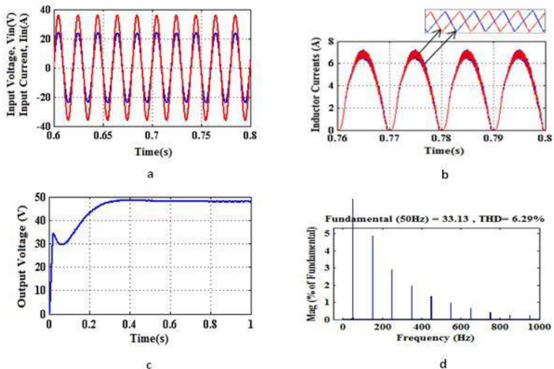
Figure-10. Simulation results of analog controlled of Interleaved Boost Converter. a. Input current and voltage in phase with each other, b. Inductor current waveforms shifted by  $180^\circ$ , c. Regulated output voltage, d. Total harmonic distortion.
