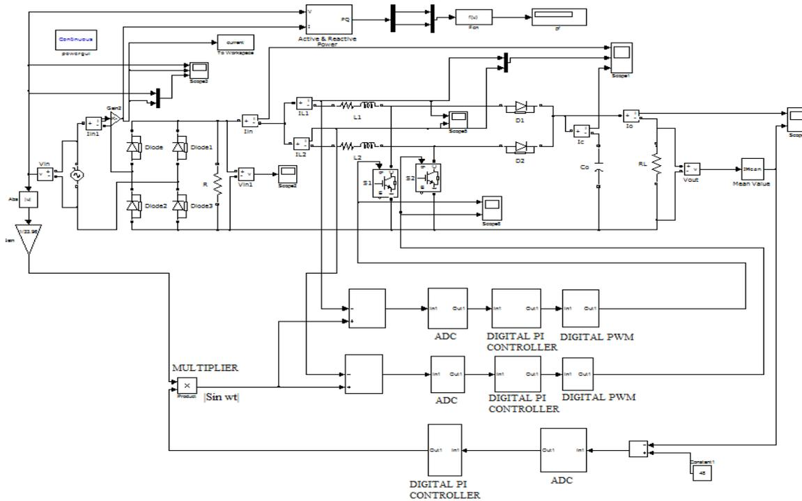
Figure-11. MATLAB/Simulink model of digitally controlled Interleaved Boost Converter.
