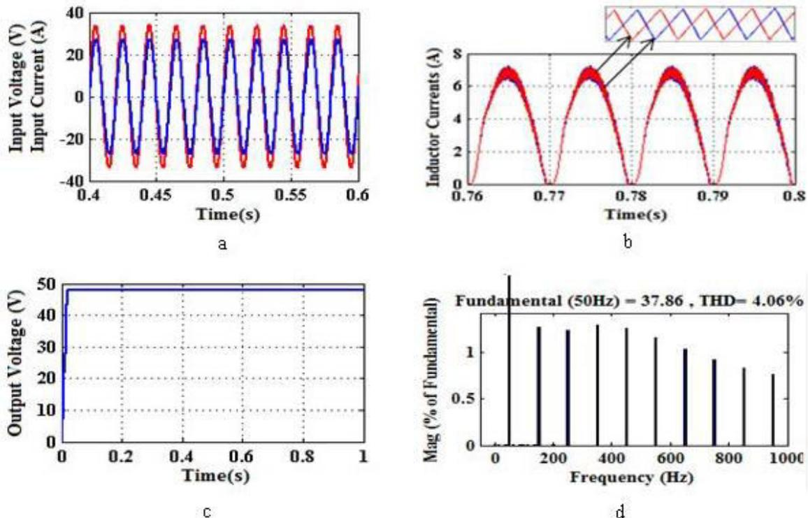
Figure-12. Simulation results of digitally controlled Interleaved Boost Converter. a. Input current and voltage in phase with each other, b. Inductor current waveforms shifted by  $180^\circ$ , c. Regulated output voltage, d. Total harmonic distortion.
