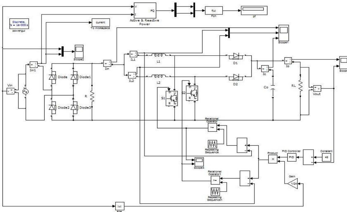
Figure-9. MATLAB/Simulink model of average current mode controlled Interleaved Boost Converter.
