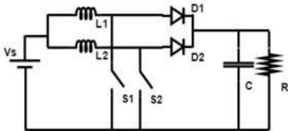
**Figure-1.** Power circuit diagram of two phase Interleaved Boost Converter.
