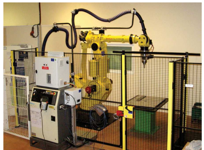
Fig. 4. RFSW test-bed incorporating a FANUC S900iB/400 RJ3iB industrial robot and an electrically driven process end-effector.
