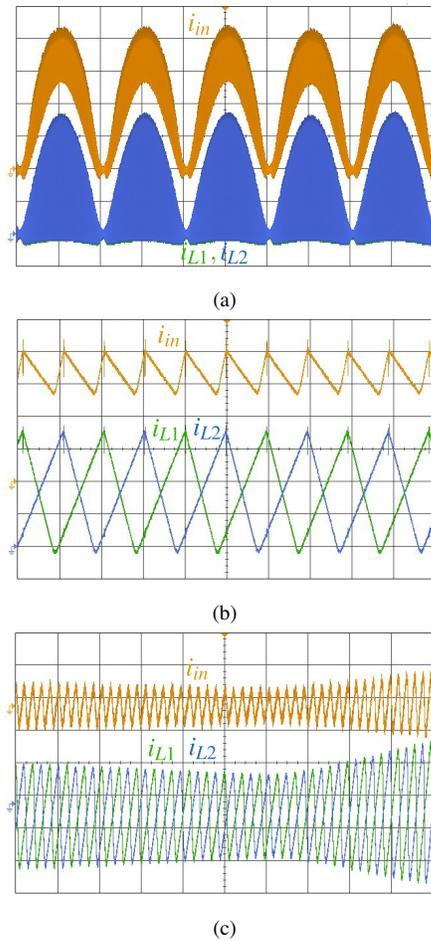
Fig. 21.  $i_{L1}$ ,  $i_{L2}$  and  $i_{in}$  when 2 boost converter channels are enabled at  $P_o = 500$  W and a rms line voltage of 115 V ( $i_{in}$ : 2 A/div,  $i_{L1}$ : 2 A/div,  $i_{L2}$ : 2 A/div). (a) Line frequency components (timebase : 5 ms/div). (b) Switching frequency components (timebase : 5  $\mu$ s/div). And (c) at the zero-crossing point of the line voltage ( $i_{in}$ : 200 mA/div,  $i_{L1}$ : 100 mA/div,  $i_{L2}$ : 100 mA/div, timebase : 20  $\mu$ s/div) .
