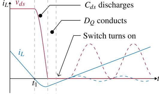
Fig. 9. Zero-voltage switching  $v_{in} < \frac{1}{2}v_o$ .
