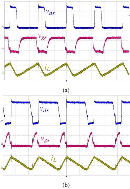
Fig. 13.  $v_{ds}$ ,  $v_{gs}$  and  $i_L$  waveforms showing valley switching for (a)  $v_{in} = 100$  V and (b)  $v_{in} = 300$  V ( $v_{ds}$ : 200 V/div,  $v_{gs}$ : 10 V/div,  $i_L$ : 2 A/div, timebase : 2  $\mu$ s/div).
