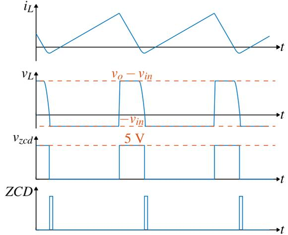
Fig. 12. Timing diagram for the ZCD generation.
