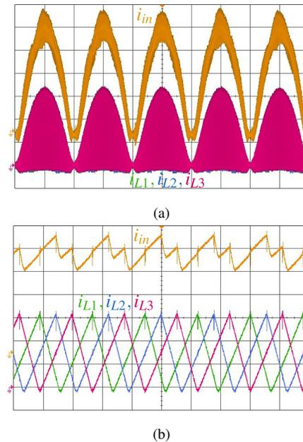
Fig. 17.  $i_{L1}$ ,  $i_{L2}$ ,  $i_{L3}$  and  $i_{in}$  when all 3 boost converter channels are enabled at  $P_o = 700$  W and a rms line voltage of 115 V when  $k_m$  is a constant gain ( $i_{in}$ : 2 A/div,  $i_{L1}$ : 2 A/div,  $i_{L2}$ : 2 A/div). (a) Line frequency components (timebase : 5 ms/div). (b) Switching frequency components (timebase : 5  $\mu s$ /div).
