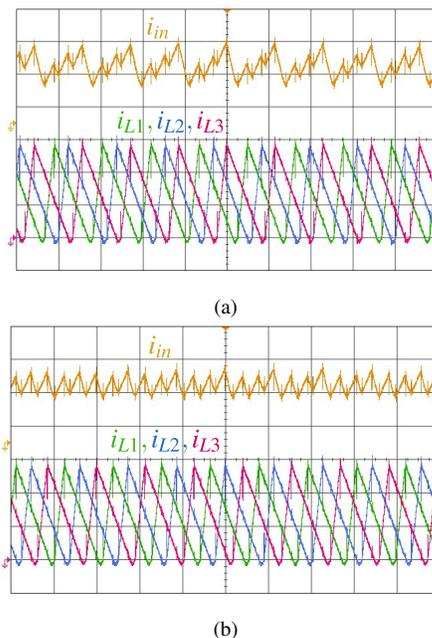
Fig. 20.  $i_{L1}$ ,  $i_{L2}$ ,  $i_{L3}$  and  $i_{in}$  when all 3 boost converter channels are enabled at  $P_o = 600$  W and a rms line voltage of 230 V ( $i_{in}$ : 2 A/div,  $i_{L1}$ : 2 A/div,  $i_{L2}$ : 2 A/div, timebase : 5  $\mu$ s/div). (a) When  $T_m$  is set to have an execution frequency of 34 kHz (b) and when  $T_m$  is set to have an execution frequency of 100 kHz.
