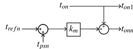
Fig. 15. Phase-shift control loop block diagram structure.
