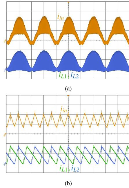
Fig. 22.  $i_{L1}$ ,  $i_{L2}$  and  $i_{in}$  when 2 boost converter channels are enabled at  $P_o = 500$  W and a rms line voltage of 230 V ( $i_{in}$ : 2 A/div,  $i_{L1}$ : 2 A/div,  $i_{L2}$ : 2 A/div). (a) Line frequency components (timebase : 5 ms/div). (b) Switching frequency components (timebase : 5  $\mu$ s/div).
