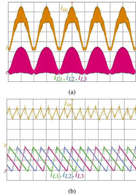
Fig. 23.  $i_{L1}$ ,  $i_{L2}$ ,  $i_{L3}$  and input current  $i_{in}$  when all 3 boost converter channels are enabled at  $P_o = 1000$  W and a rms line voltage of 230 V ( $i_{in}$ : 2 A/div,  $i_{L1}$ : 2 A/div,  $i_{L2}$ : 2 A/div). (a) Line frequency components (timebase : 5 ms/div). (b) Switching frequency components (timebase : 5  $\mu$ s/div).
