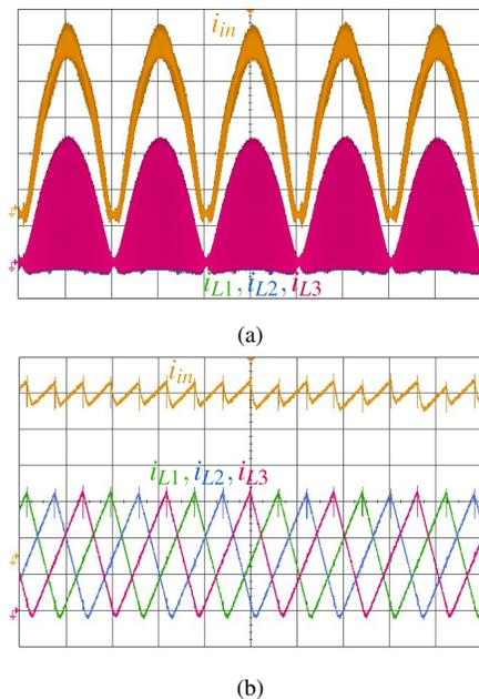
Fig. 19.  $i_{L1}$ ,  $i_{L2}$ ,  $i_{L3}$  and  $i_{in}$  when all 3 boost converter channels are enabled at  $P_o = 700$  W and a rms line voltage of 115 V when  $k_m$  is an adaptive gain ( $i_{in}$ : 2 A/div,  $i_{L1}$ : 2 A/div,  $i_{L2}$ : 2 A/div). (a) Line frequency components (timebase : 5 ms/div). (b) Switching frequency components (timebase : 5  $\mu$ s/div).
