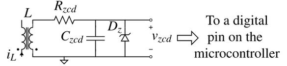
Fig. 11. Zero-current-detection circuit.
