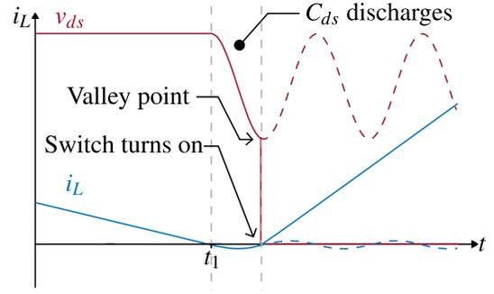
Fig. 10. Near-zero-voltage switching  $v_{in} > \frac{1}{2}v_o$ .
