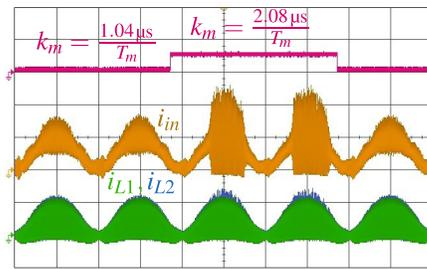
Fig. 16. Input current  $i_{in}$  and inductor currents  $i_{L1}$  and  $i_{L2}$  when the gain  $k_m$  is toggled from a value of  $k_m = \frac{1.04 \mu s}{T_m}$  to a value of  $k_m = \frac{2.08 \mu s}{T_m}$  at  $P_o = 225$  W,  $t_{on} = 0.9 \mu s$  and a rms line voltage of 200 V. ( $i_{in}$ : 2 A/div,  $i_{L1}$ : 2 A/div,  $i_{L2}$ : 2 A/div, timebase : 5 ms/div).
