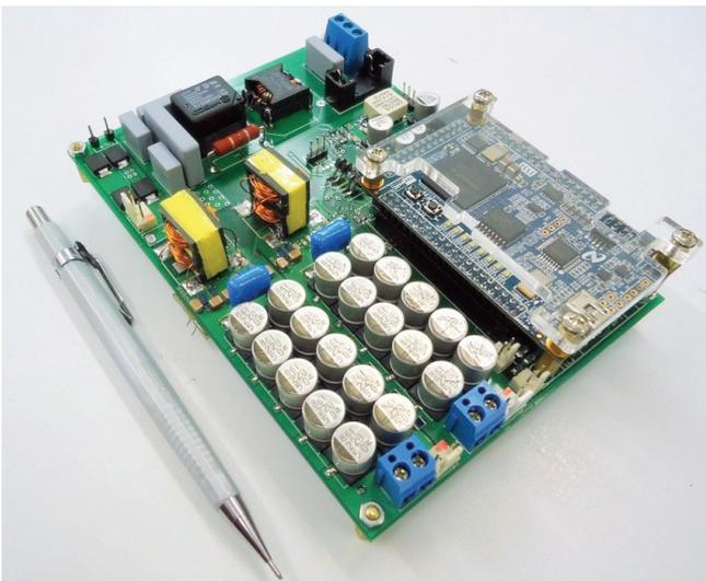
Fig. 4. : Hardware implementation of fully digital high switching frequency single-phase interleaved boost-type PFC rectifier.
