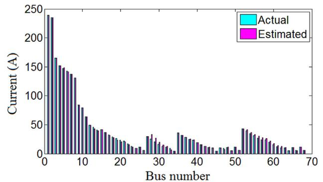
Fig. 15. Complete branch currents, 69-bus feeder, test case #24.
