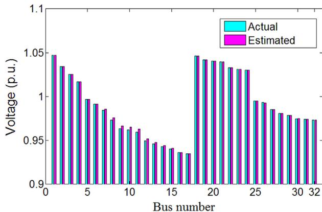
Fig. 10. Complete voltage profile, 33-bus feeder, test case #4.
