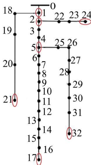
Fig. 7. Layout of the 33-bus feeder following SM placement.
