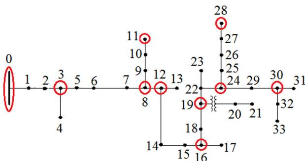
Fig. 9. Layout of the 34-bus feeder after SMs placement.
