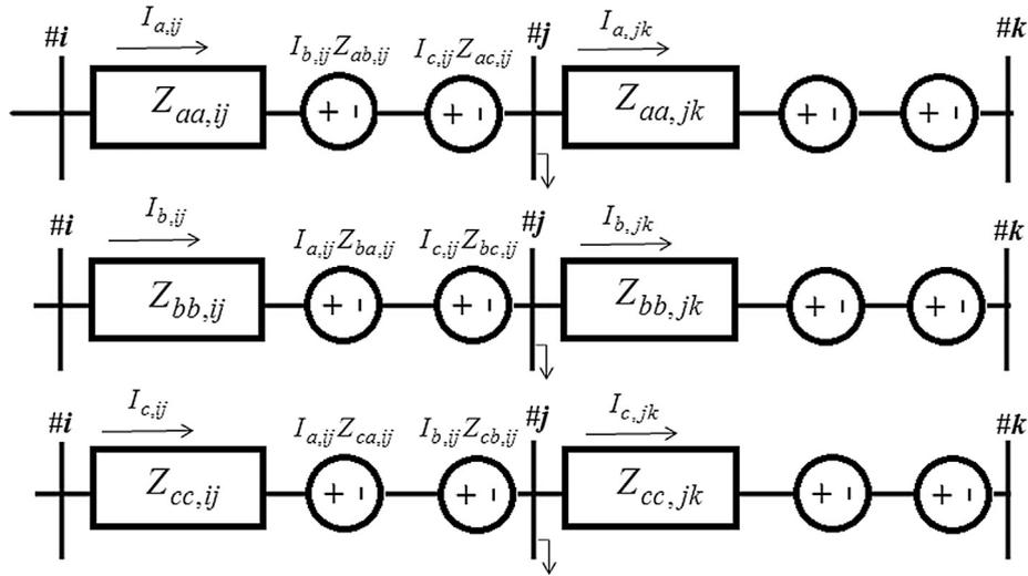
Fig. 3. Three phase equivalent circuit of branch.
