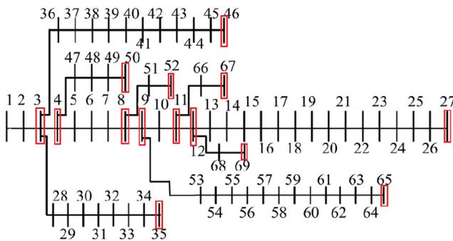
Fig. 8. Layout of the 69-bus feeder following SM placement.
