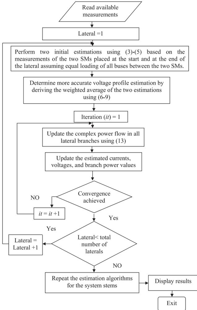
Fig. 4. Flow chart of the proposed algorithms.
