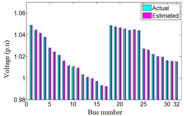
Fig. 11. Complete voltage profile, 33-bus feeder, test case #12.
