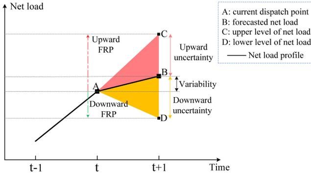
Fig. 1 Illustration of system-wide ramping capability requirement
