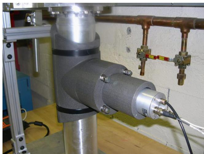
**Fig. 4.** Detector shield made of tungsten powder in a special polymer.
