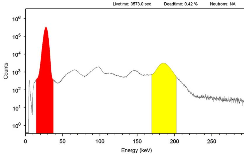
**Fig. 7.** Spectrum measured with the new enrichment monitor design when the pipe contains 6.67 kPa of UF<sub>6</sub>. The 25-keV transmission peak is produced by the X-ray tube with a silver filter. The 186-keV peak is from <sup>235</sup>U.
