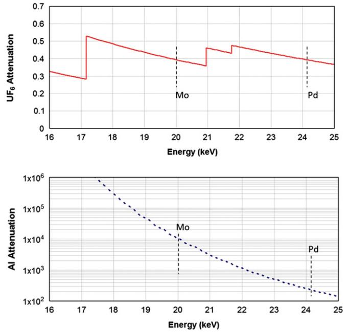
Fig. 5. Attenuation as a function of energy in  $\text{UF}_6$  gas (top) and an Al pipe with 100 mm ID and 110 mm OD (bottom). Note the log scale on the Al attenuation. The energies of the molybdenum and palladium X-ray K edges are indicated.
