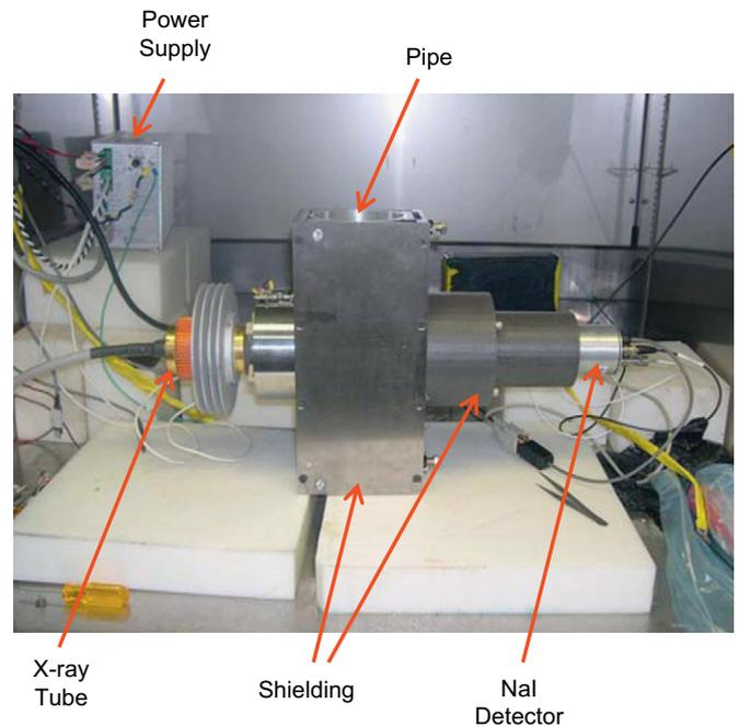
Fig. 6. A laboratory version of an enrichment monitor that includes all of the techniques discussed in this report. In this setup, the pipe does not contain gas.
