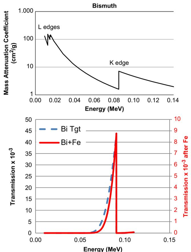
Fig. 2. Top: bismuth photon mass attenuation coefficient. Bottom: calculated photon spectrum incident on the pipe (dashed line) and after passage through the pipe (solid line).
