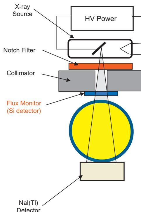
**Fig. 3.** Schematic of the transmission system showing the filter and flux monitor.
