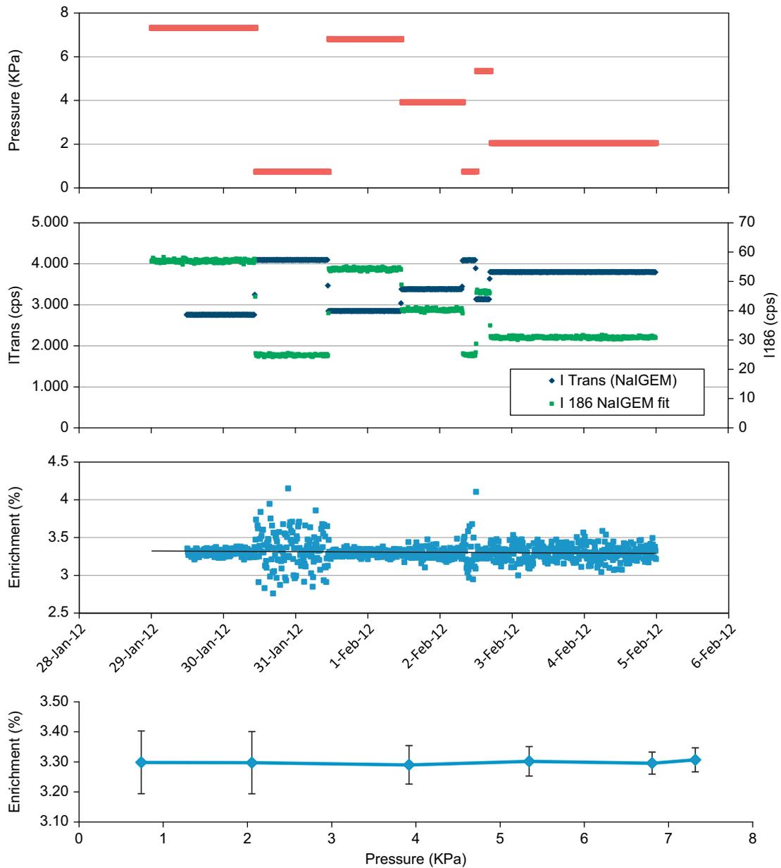
**Fig. 8.** Performance of the enrichment monitor when the pressure is changed. The top chart shows the pressure vs. date. The second chart shows the 122-keV transmission peak and the 186-keV peak counting rates vs. date. The third chart shows the <sup>235</sup>U enrichment vs. date. The fourth chart shows the <sup>235</sup>U enrichment vs. pressure.
