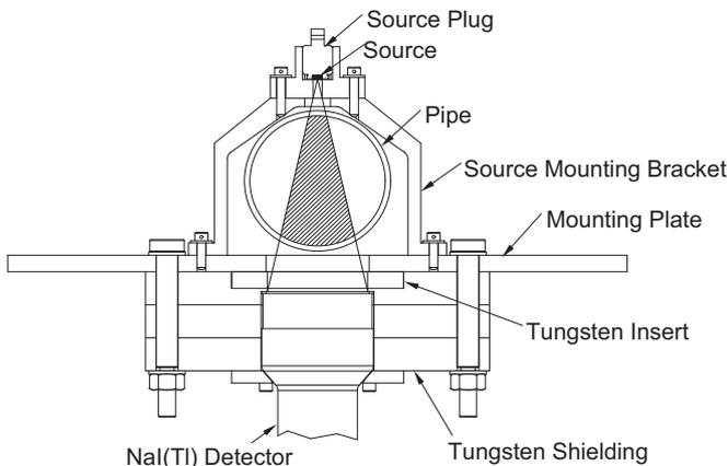
Fig. 1. Cross section of the original transmission design for the enrichment monitor.
