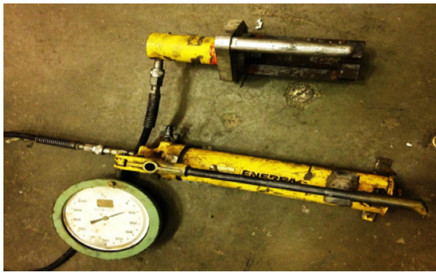
Fig. 4. Hydraulic manual pump and jack used in pre-seating the anchor.
