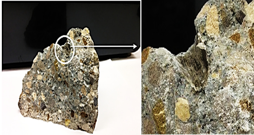
Fig. 10. Adherence of sand coating of basalt bars to the concrete surface.
