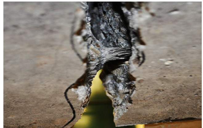
Fig. 9. Sand coating sheared off the basalt bars.
