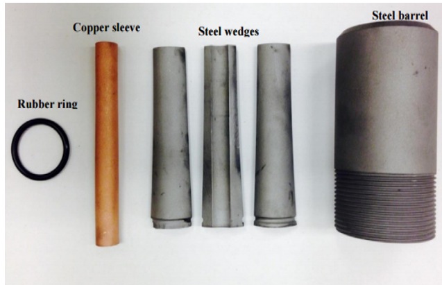
Fig. 3. Anchorage components used for prestressing.
