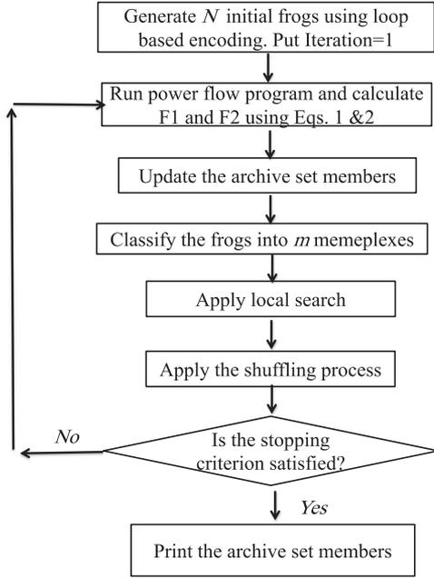
Fig. 1. The flowchart of algorithm.
