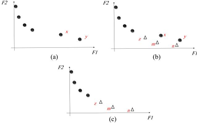
Fig. 3. Updating the archive set members. Circles: The AS members at Iteration T Triangles: The new identified AS members (a) AS at Iteration T (b) Adding the new non-dominated frogs (c) Removing the dominated frogs.
