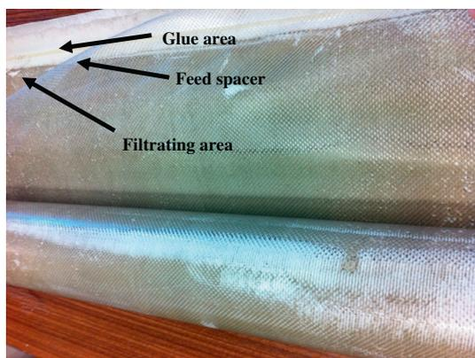
Fig. 4. Inside image of the 1st NF270 module.
