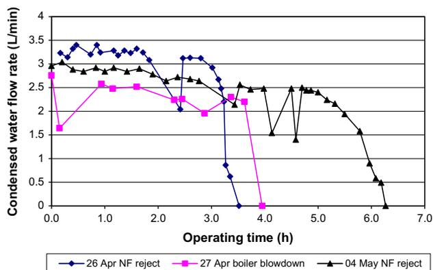
Fig. 6. Condensed distillate flow rate profiles for the three evaporator tests.
