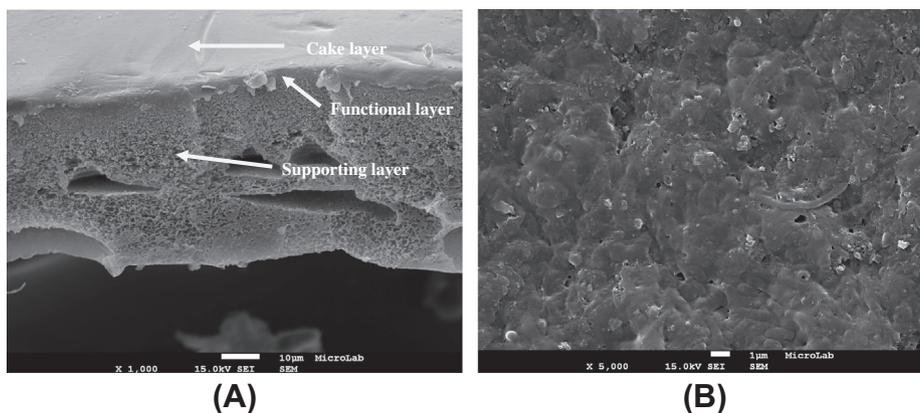
Fig. 5. SEM image of the first NF270. SEM image of cross-section (A) and membrane surface (B).
