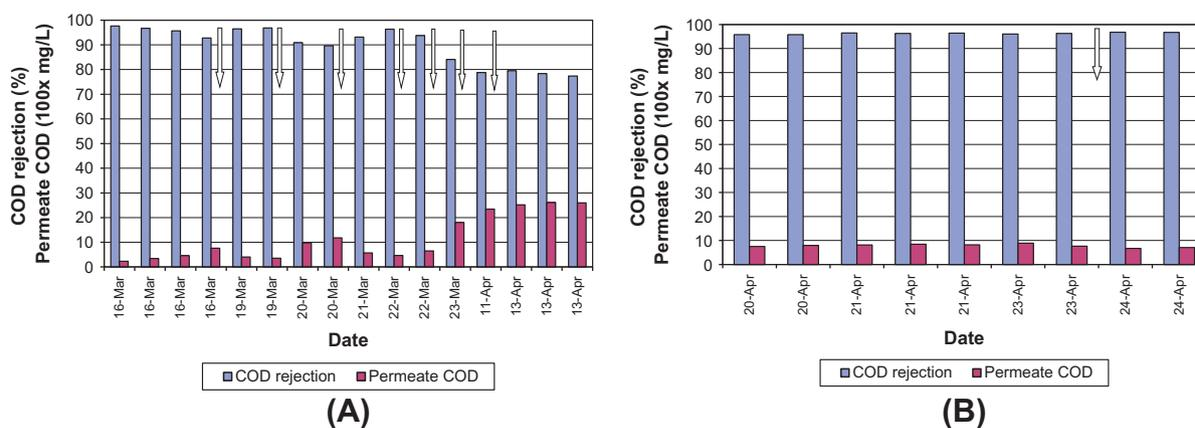
**Fig. 3.** COD rejection and permeate COD values for the first membrane (A) and the second membrane (B) with the rubber wastewater as feed water. White arrows indicate when chemical cleanings were carried out.
