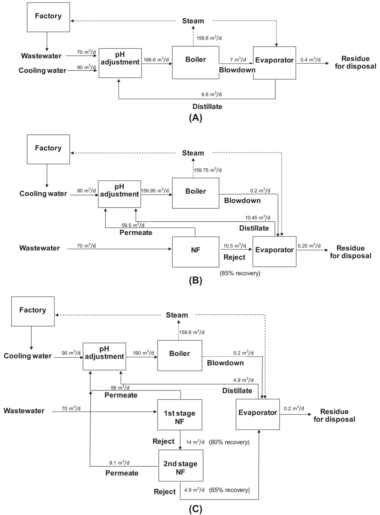
Fig. 7. Mass balance of the existing process (A), the single stage NF + evaporator (B) and the two-stage NF + evaporator design (C).
