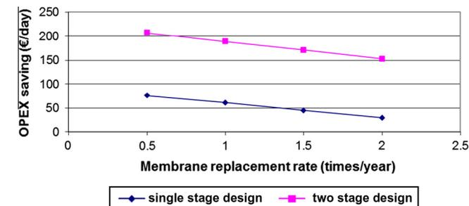
Fig. 8. OPEX savings at different membrane replacement rates (85% water recovery is assumed for the single stage design; 80% and 65% water recoveries are assumed for the first and second stages in the two-stage design).
