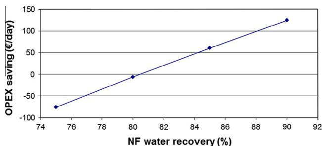
Fig. 9. OPEX savings at different water recoveries for the single stage NF design (the membrane replacement rate is assumed once per year).
