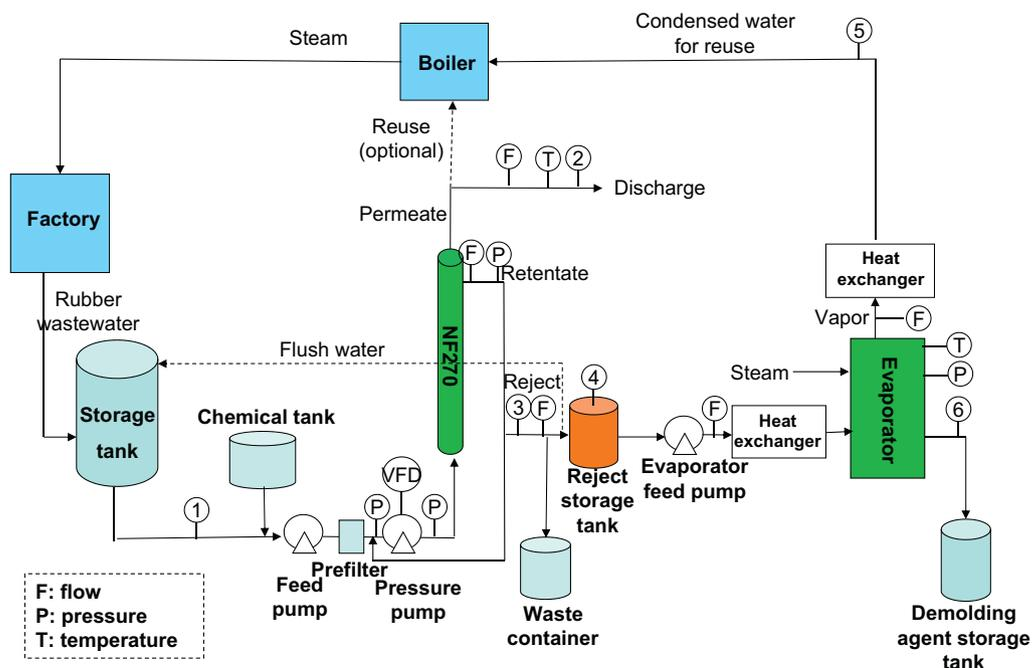
Fig. 1. Schematic process diagram of the pilot system at Cikautxo. Sensors for flow, pressure and temperature are labelled as F, P and T, respectively. Sampling locations are numbered. VFD: variable frequency drive.
