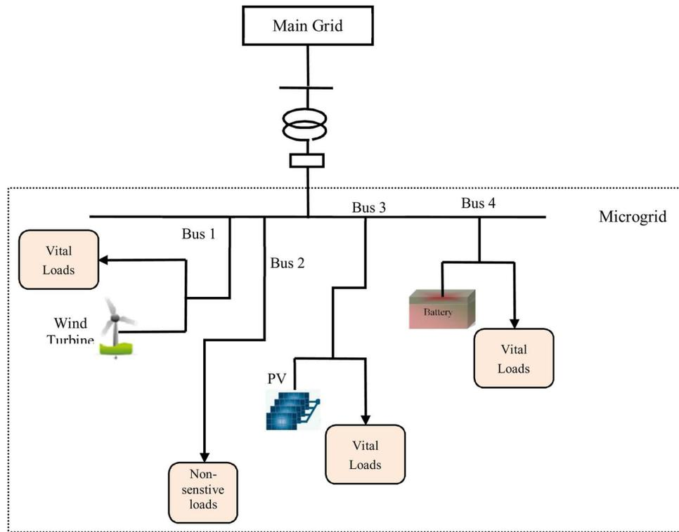
Fig. 4. Microgrid architecture.
