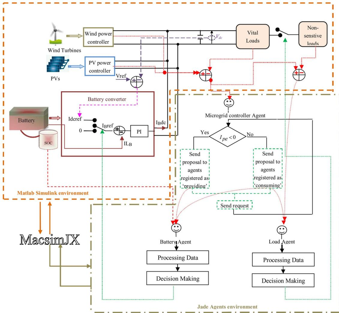
Fig. 9. Microgrid control by MAS.
