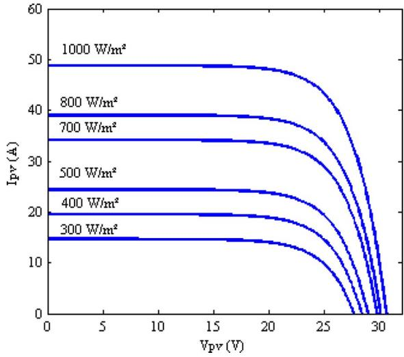
Fig. 3. I-V characteristic curves of the PV modules at different irradiances.
