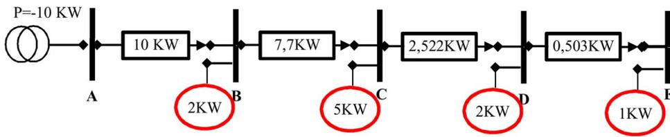
Fig. 11. The transit power in the line without DG.
