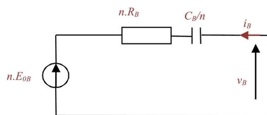
Fig. 6. The battery model of n cell.
