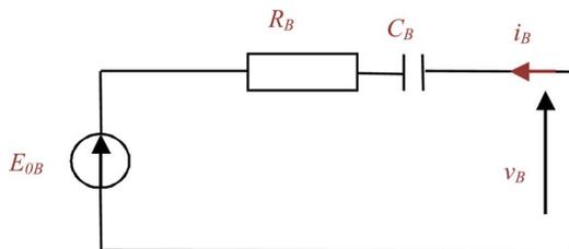
Fig. 5. The proposed battery model.
