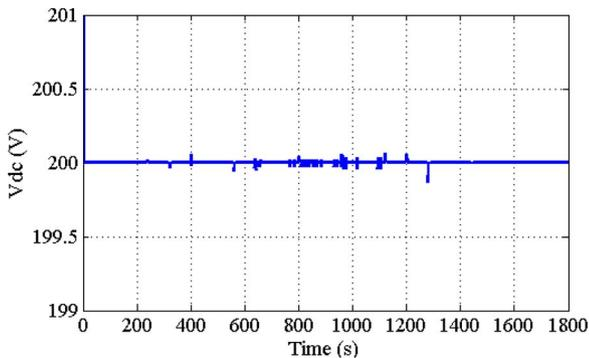
Fig. 18. Microgrid DC bus voltage during simulation.
