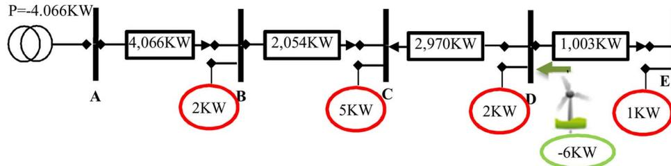
Fig. 12. The transit power with one DG ( $P_w = 6KW$ ).
