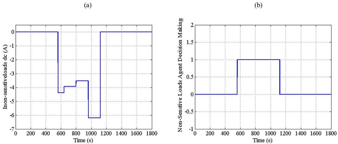
Fig. 16. (a) Non-sensitive loads Agent reaction in the DC bus, (b) Non-sensitive loads Agent decision making.
