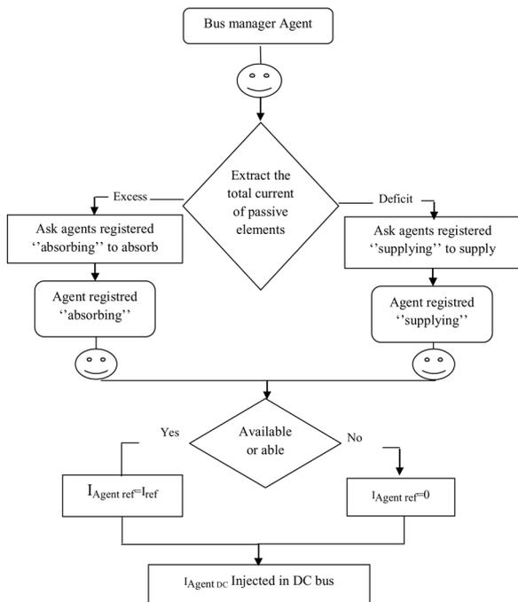
Fig. 10. General algorithm of EMS in a microgrid using MAS.
