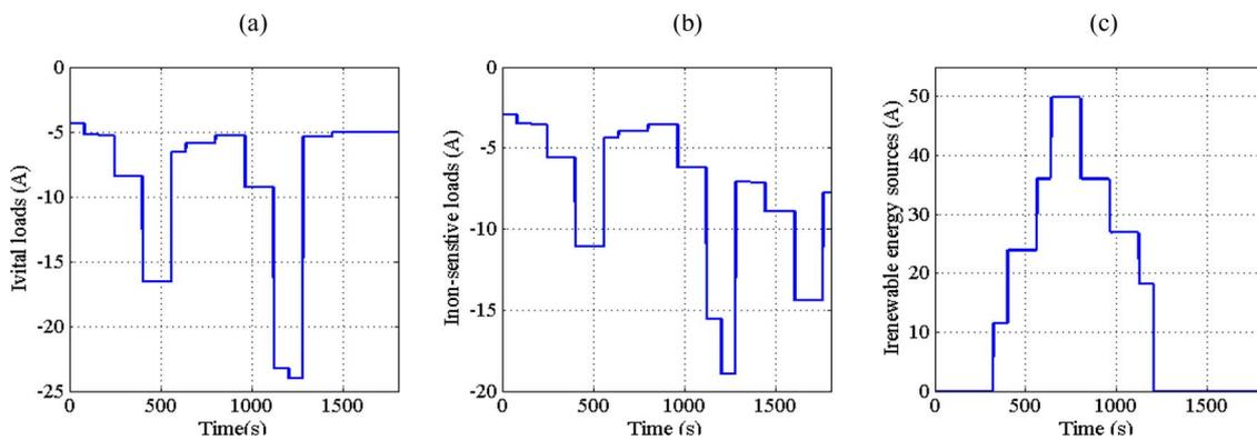
Fig. 15. (a) Vital loads consumption, (b) Non sensitive loads consumption (c) RES production.
