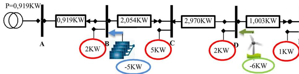
Fig. 13. The transit power with one DG ( $P_w = 6KW$ ,  $P_{pv} = 5KW$ ).
