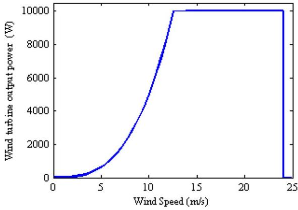
Fig. 2. Wind turbine output power characteristic vs wind speed.
