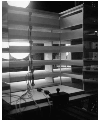
Fig. 5. Detail of the variable glazing surface.
