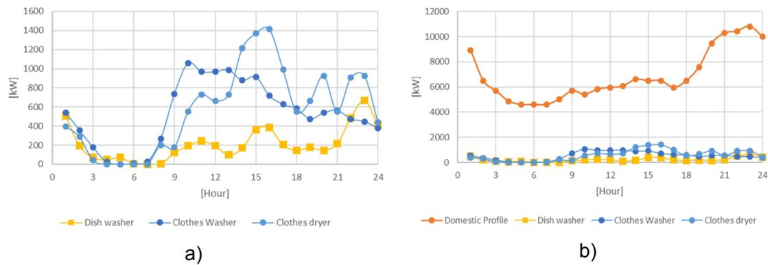
Fig. 3. a) Domestic equipment load profiles; b) Equipment's share in the island's domestic sector load.
