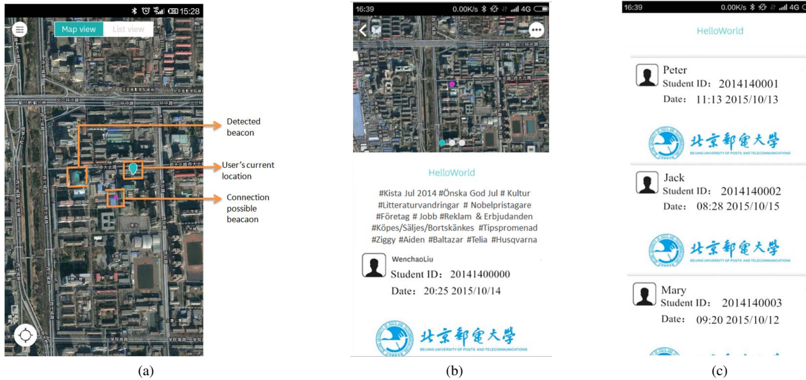
Fig. 6. Example of laboratory check-in service. (a) Information prompting a student to check-in when near the door. (b) Information on the student's mobile phone after check-in. (c) Check-in list visible for a professor.
