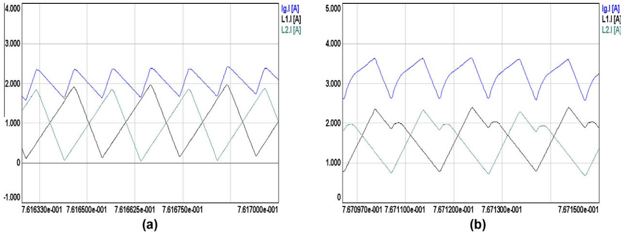
Fig. 8. Simulation results of (a)  $i_{L1}-i_{L2}-i_g$  (for  $d > 0.5$ ) and (b)  $i_{L1}-i_{L2}-i_g$  (for  $d < 0.5$ ).
