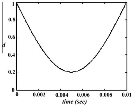
Fig. 2. Variation of the duty cycle ( $d$ ) for PFC circuits.
