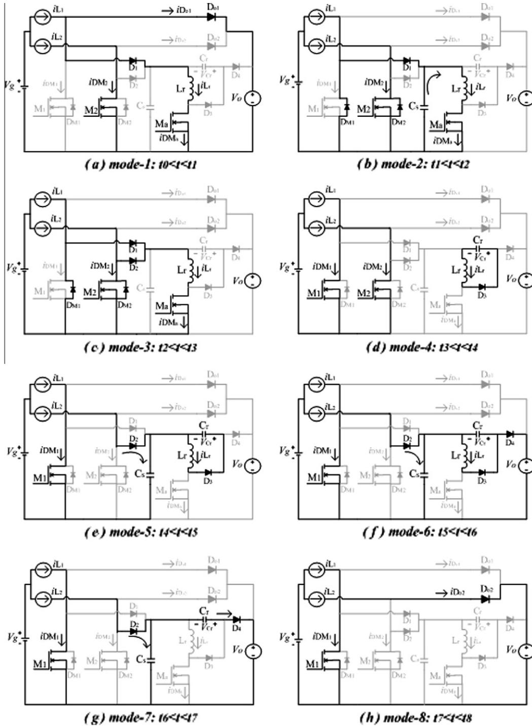
Fig. 5. Equivalent circuits corresponding to different operating modes (for  $d > 0.5$ ).
