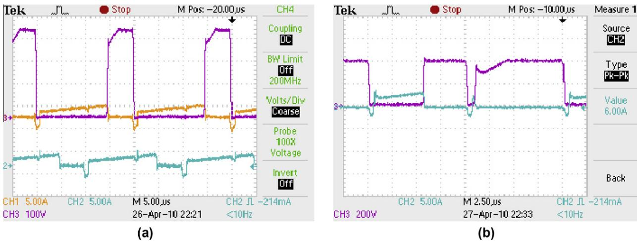
Fig. 15. Experimental results of (a)  $V_{DSM1}$ ,  $i_{DM1}$ ,  $i_{DM2}$  (for  $d > 0.5$ ) and (b)  $V_{DSM1}$ ,  $i_{DM1}$  (for  $d < 0.5$ ).
