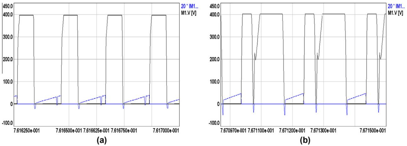
Fig. 9. Simulation results of (a)  $V_{DSM1}, 20 * i_{DM1}$  (for  $d > 0.5$ ) and (b)  $V_{DSM2}, 20 * i_{DM2}$  (for  $d < 0.5$ ).
