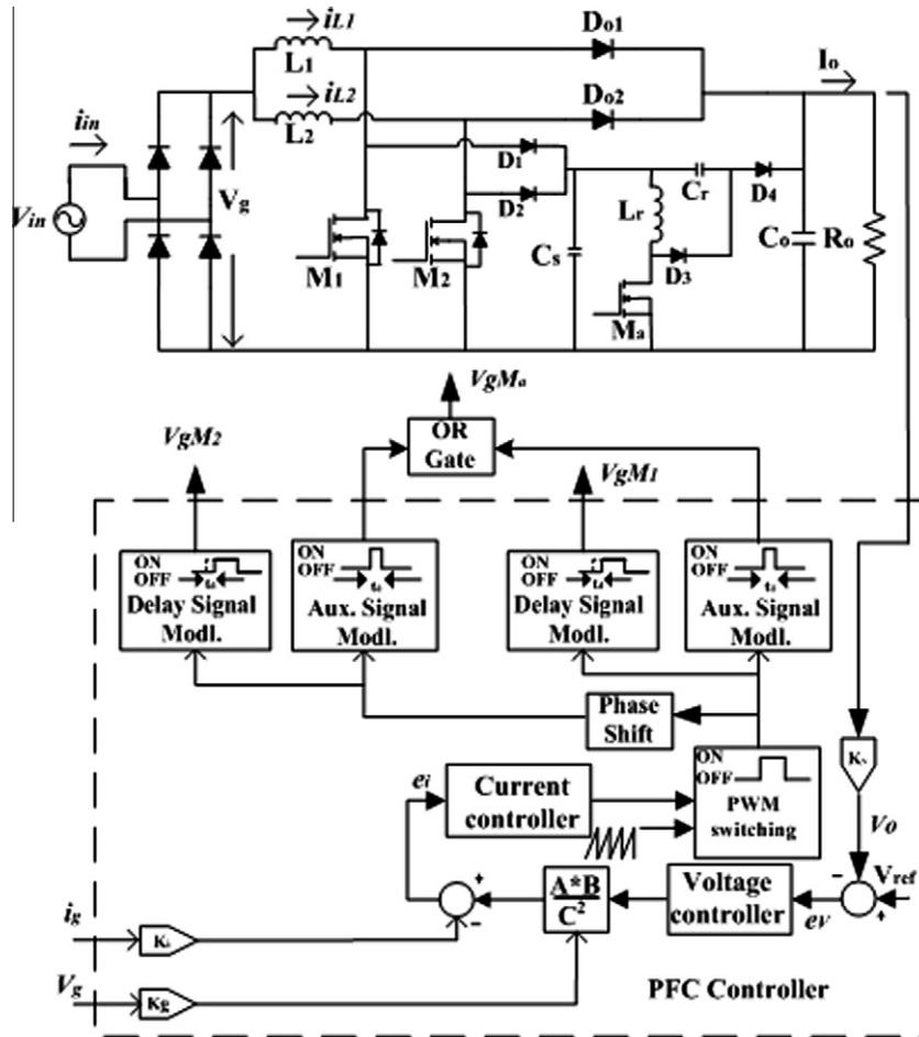
Fig. 6. The scheme of controller and power stage of the proposed topology.
