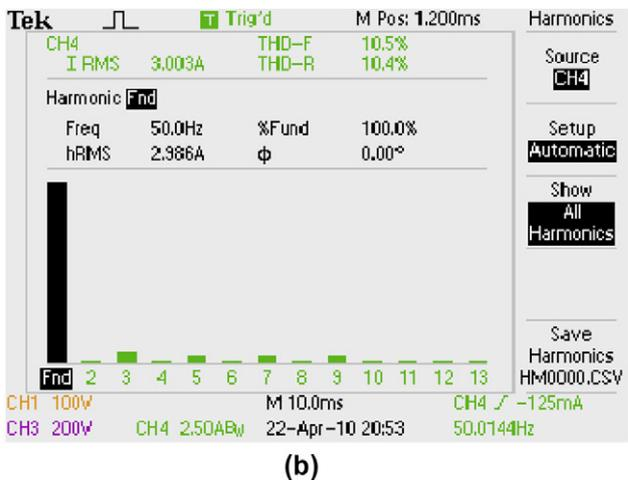
**Fig. 11.** Experimental results of (a) input voltage ( $V_{in} = 220 V_{rms}$ ) and input current ( $i_{in} = 2.98 A_{rms}$ ) and (b) harmonic analysis of input current (THD = 10.4%, pf = 0.994).
