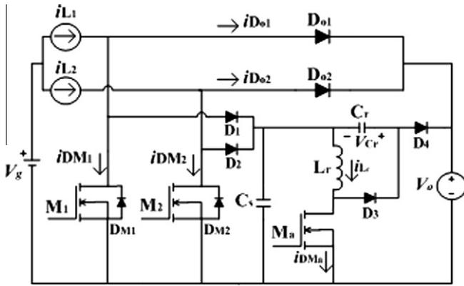
Fig. 3. Simplified circuit diagram of the proposed topology.
