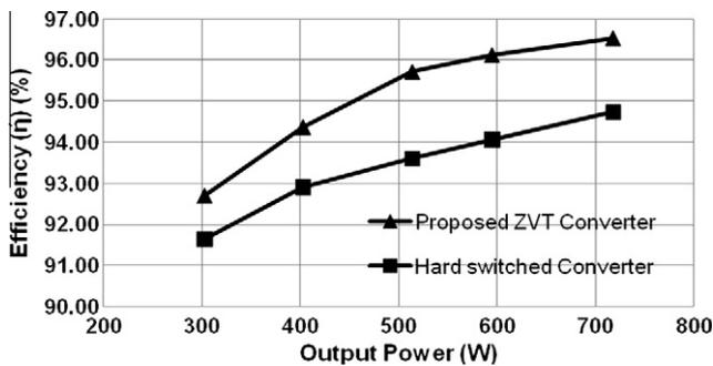
Fig. 17. Experimental efficiency comparison of the proposed ZVT interleaved boost PFC converter and conventional hard switched interleaved boost PFC converter.
