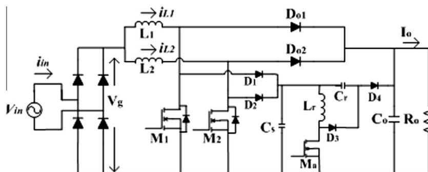
Fig. 1. The proposed ZVT two cell interleaved boost PFC converter.
