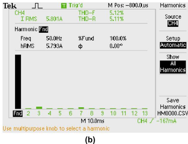
**Fig. 12.** Experimental results of (a) input voltage ( $V_{in} = 110 V_{rms}$ ) and input current ( $i_{in} = 5.80 A_{rms}$ ) and (b) harmonic analysis of input current (THD = 5.1%, pf = 0.998).
