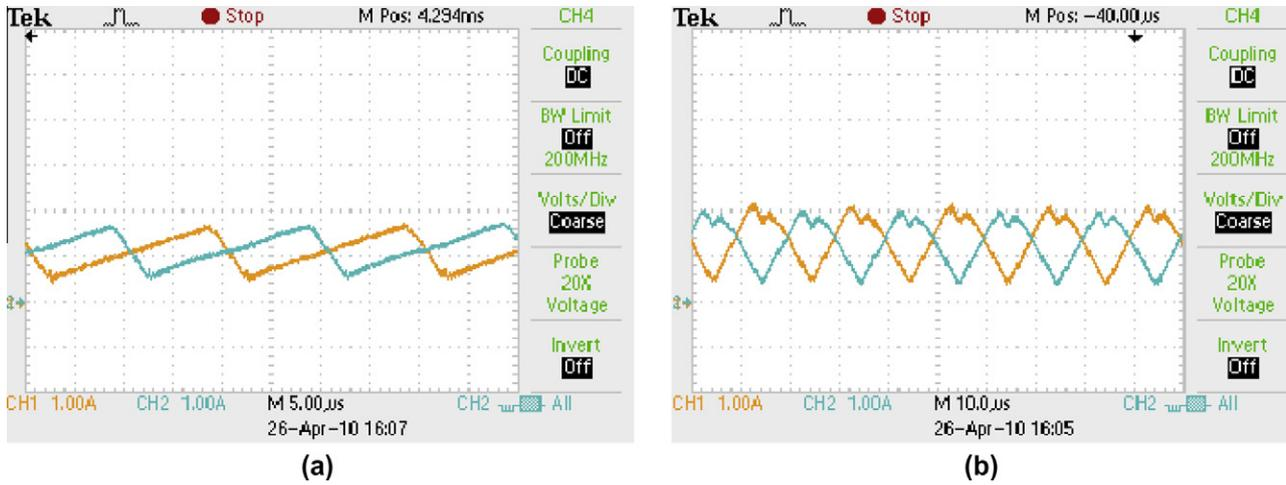
Fig. 13. Experimental results of (a)  $i_{L1}-i_{L2}$  (for  $d > 0.5$ ) and (b)  $i_{L1}-i_{L2}$  (for  $d < 0.5$ ).
