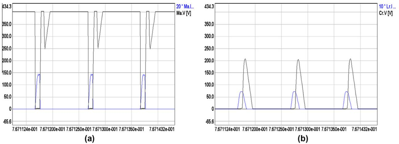
Fig. 10. Simulation results of (a)  $V_{DSMa}, 20 * i_{DMa}$  and (b)  $V_{Cr}, 10 * i_{Lr}$ .
