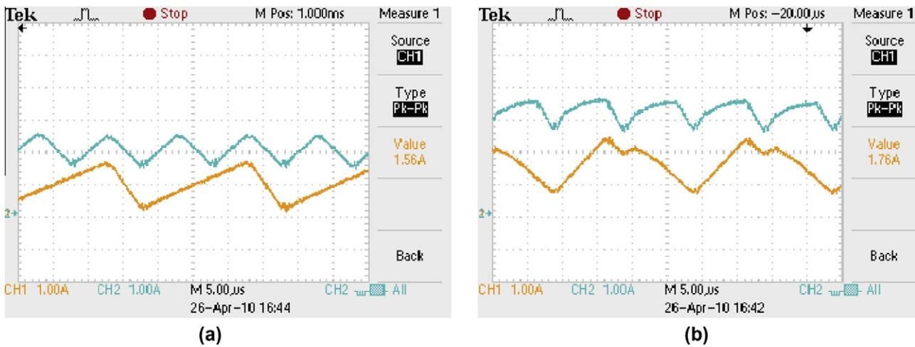
Fig. 14. Experimental results of (a)  $i_{L1}-i_g$  (for  $d > 0.5$ ) and (b)  $i_{L1}-i_g$  (for  $d < 0.5$ ).
