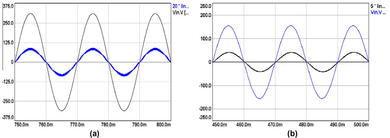
Fig. 7. Simulation results of (a) input voltage ( $V_{in} = 220 V_{rms}$ ) and  $20 \times$  input current ( $i_{in} = 2.77 A_{rms}$ ) and (b) input voltage ( $V_{in} = 110 V_{rms}$ ) and  $5 \times$  input current ( $i_{in} = 5.59 A_{rms}$ ) waveforms.
