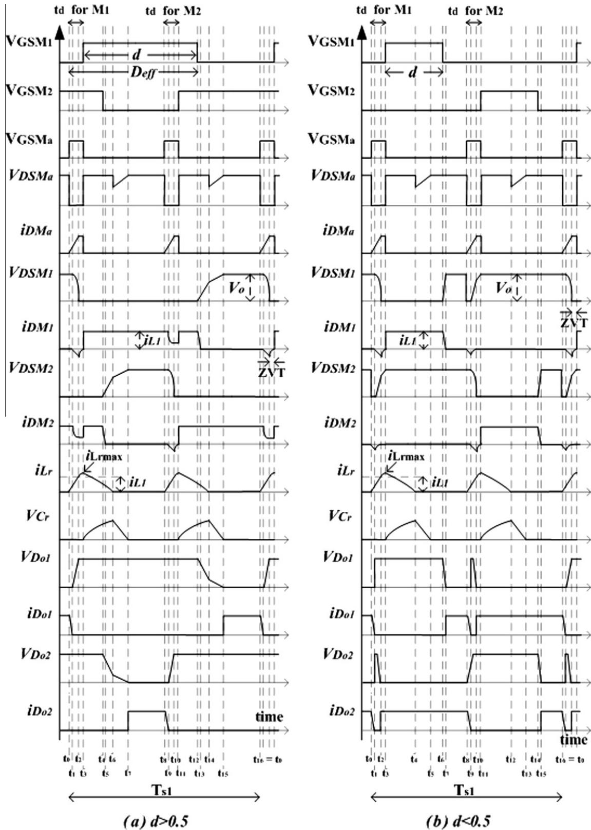
Fig. 4. Theoretical waveforms of the proposed topology (for  $d > 0.5$  and  $d < 0.5$ ).
