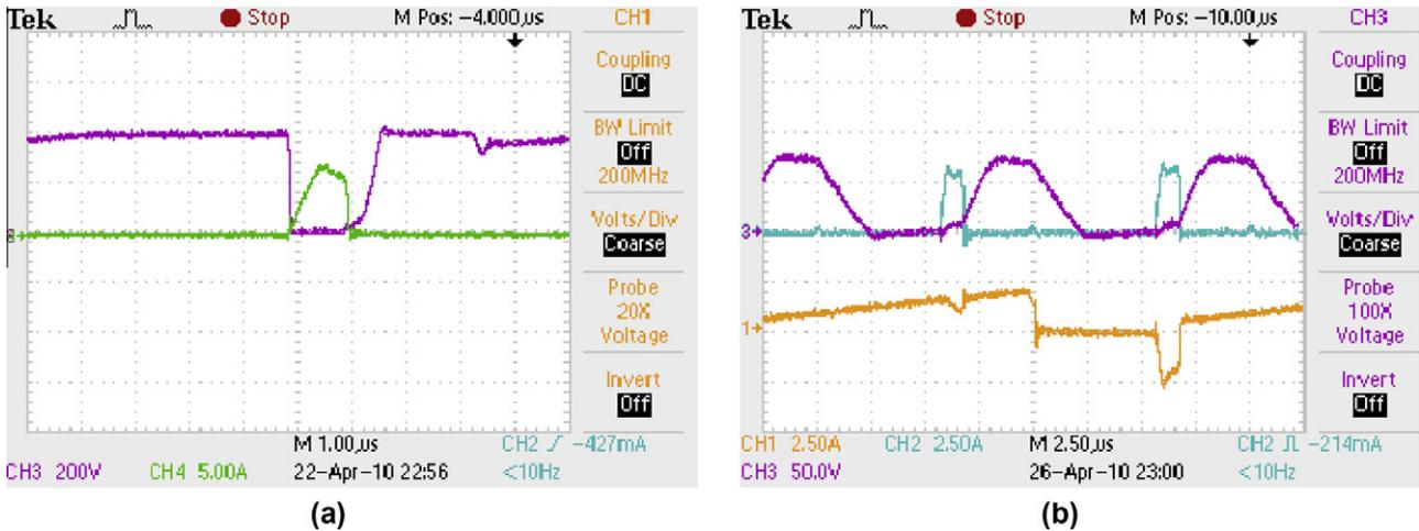
Fig. 16. Experimental results of (a)  $V_{DSMa}$ ,  $i_{DMa}$  and (b)  $V_{Cr}$ ,  $i_{DM1}$ ,  $i_{DMa}$ .
