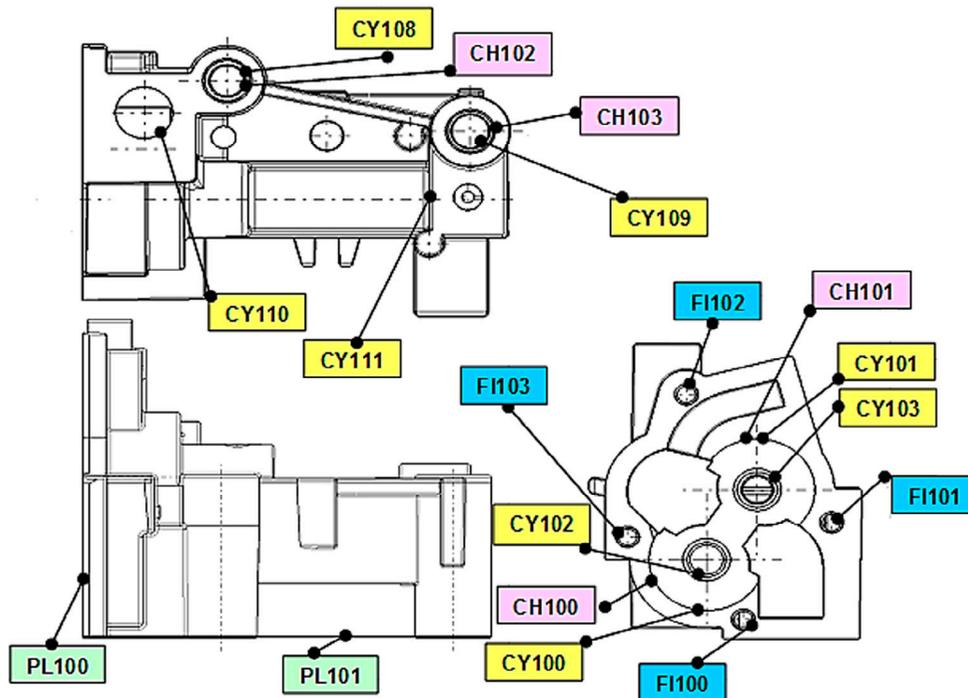
Figure 7. Labelled operations of the industrial part.
