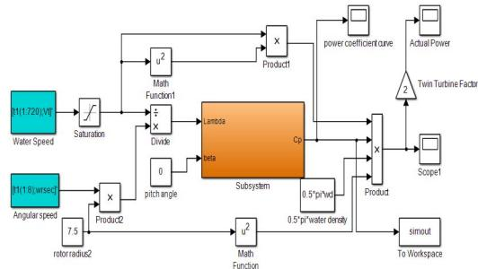
Figure 5 Simulink model of the Tidal Current Turbine
