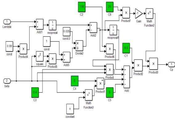
Figure 4 Simulink model of the power coefficient
