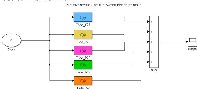
Figure 3 Model of the Tidal current velocity profile
