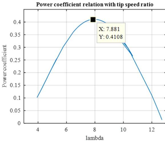
Figure 7 Power coefficient relation with tip speed ratio
