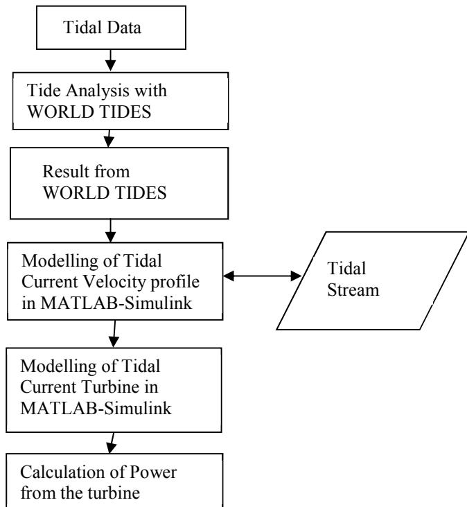
Figure 1: Block Diagram of the Proposed Design
