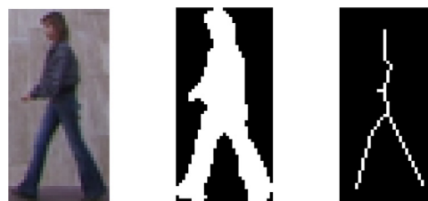
Fig. 1. A frame of the sequence (a); binary image where the foreground is the silhouette (b); the graph obtained by skeletonization and polygonal approximation (c).
