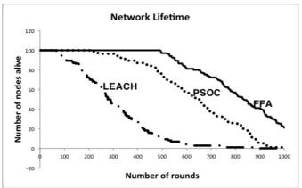
Fig. 3:Network lifetime for the nodes with uniform energy
