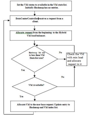
Fig.1 Flowchart for Hybrid VM load balancer
