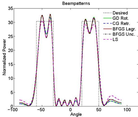
(a) beampatterns after 20 iterations
