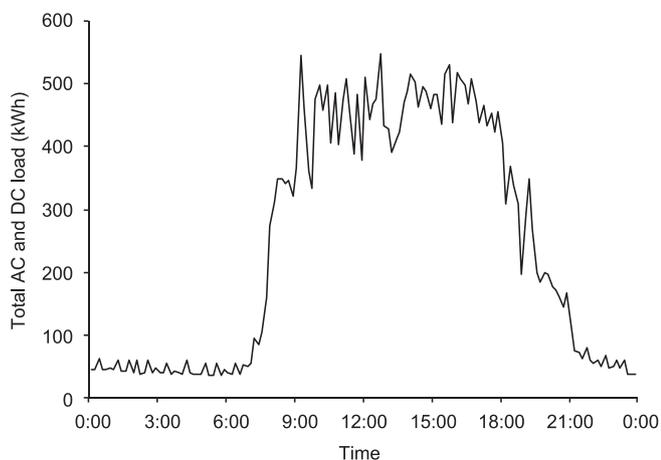
Fig. 5. Total AC and DC load measured every 10 min during a day (kWh).
