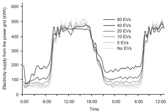
**Fig. 8.** Electricity supply from the power grid for every 10 min with different numbers of EVs (kWh).
