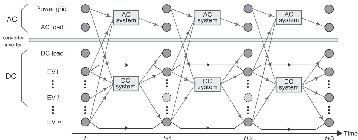
Fig. 2. Time-space network model for the local electric power network.
