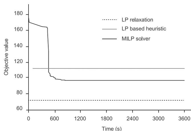
**Fig. 9.** Time courses of the objective values for the LP based heuristic algorithm and the MILP solver with 80 EVs.
