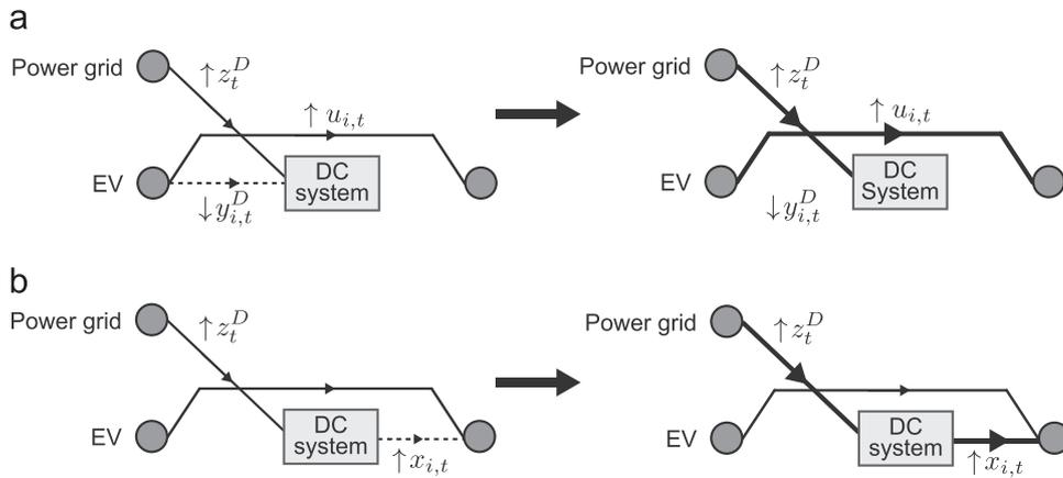
Fig. 3. Rounding procedures of the LP based heuristic algorithm: (a) rounding down  $y_{i,t}^A$  and  $y_{i,t}^D$  to zero and (b) rounding up  $x_{i,t}$  to one.
