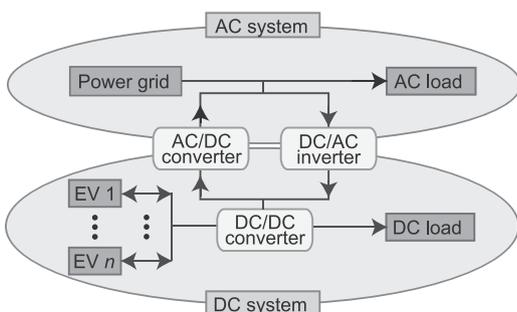
Fig. 1. Local electric power network of the BEMS.
