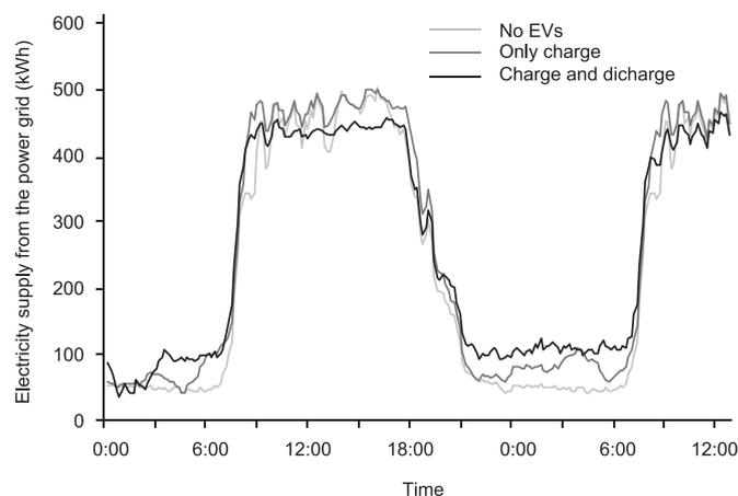
Fig. 6. Electricity supply from the power grid for every 10 min (kWh).
