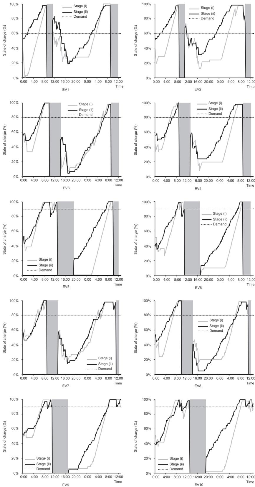
Fig. 7. State of charge for EV1–10 obtained with the smart charge and discharge schedules.
