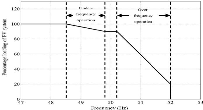
Figure 5: Variation of PV system power with frequency deviation
