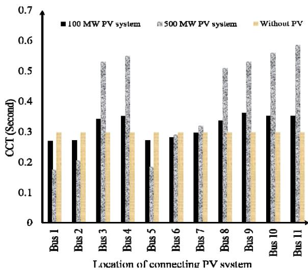
Figure 12: CCT with connecting PV system at different locations
