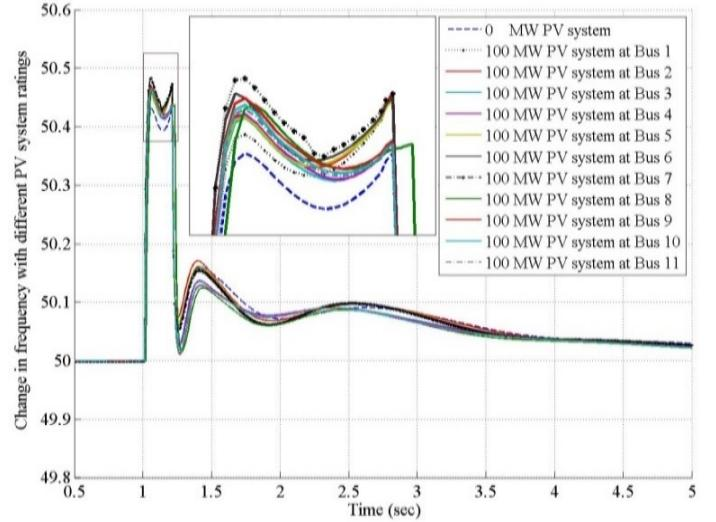
Figure 10: Frequency variation with connecting PV unit at all busses
