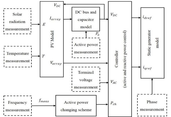
Figure 2: Composed model for PV system in DigSILENT
