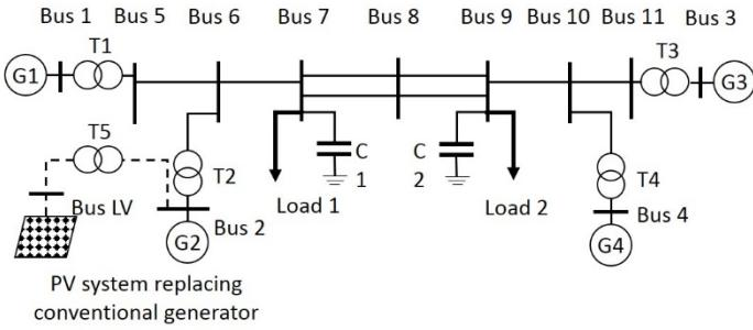
Figure 6: Four-machine, 11-bus power system
