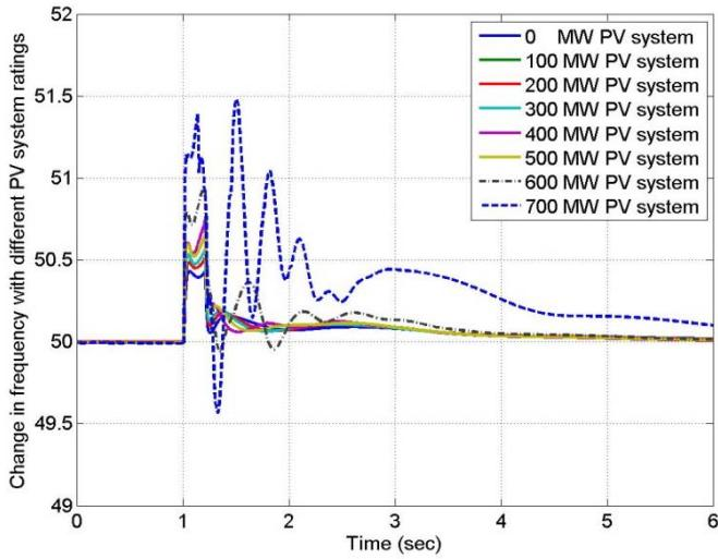
Figure 9: Frequency variation with replacing G2 by PV units
