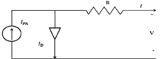
Figure 3: Equivalent circuit of a solar PV cell
