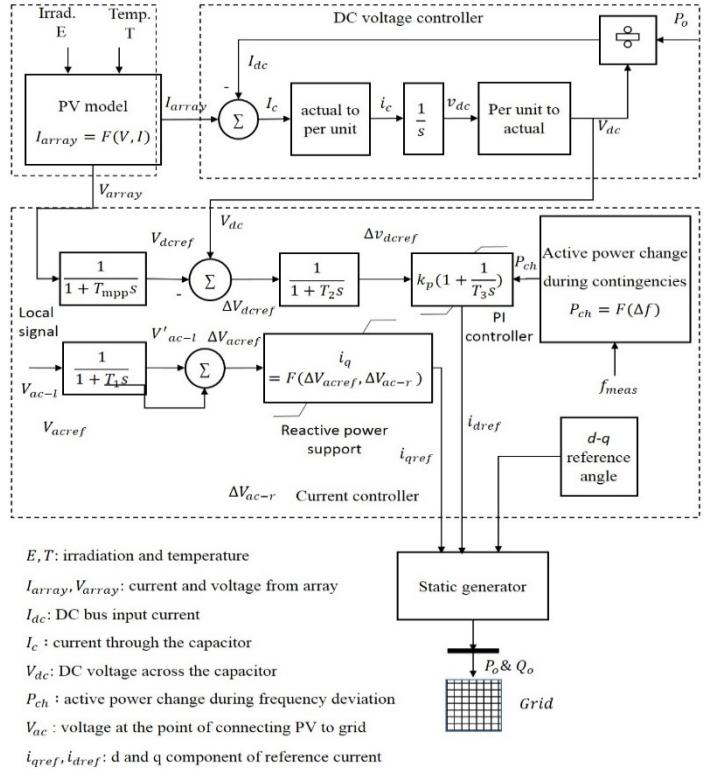
Figure 4: Control loops in PV system composite model
