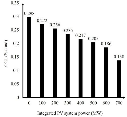
Figure 7: CCT with replacing G2 by PV system units
