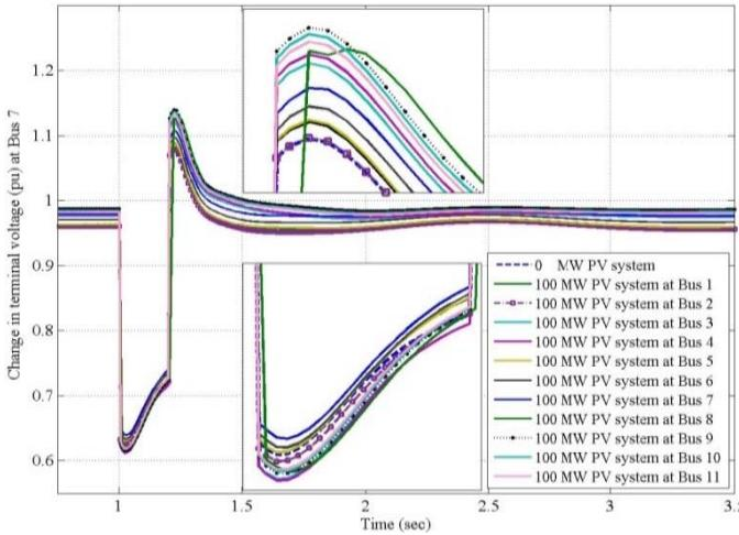
Figure 11: The terminal voltage at bus 7
