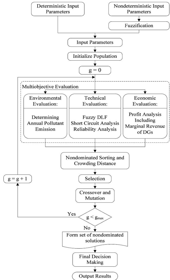
Fig. 1. Proposed algorithm for distributed generation expansion planning.
