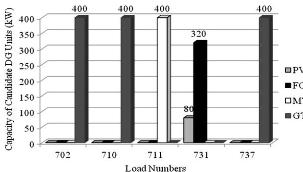
Fig. 7. Size, location and technology of DG units in the optimal planning scheme in scenario B.
