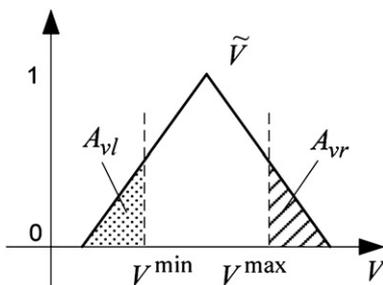
Fig. 3. Fuzzy voltage constraint modeling as a risk value.
