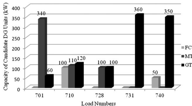
**Fig. 9.** Size, location and technology of DG units in the optimal planning scheme in scenario C.
