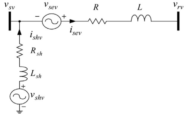
Fig. 2. Single phase representation of the UPFC system.
