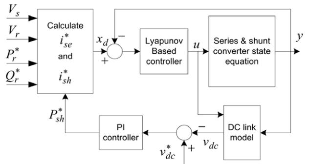
Fig. 4. Block diagram of the overall UPFC control system.
