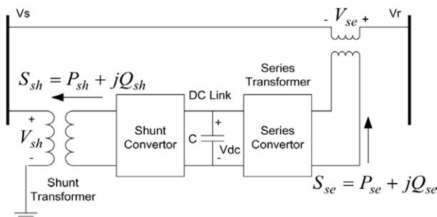
Fig. 1. Schematic diagram of the UPFC system.
