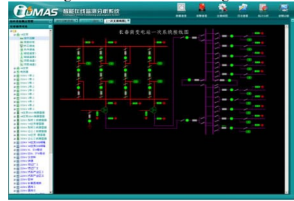
Fig.10 interface showing the status of the primary equipment being monitored
