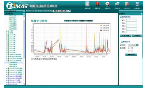
Fig.11 interface showing the diagnosis result of insulation parameters by comparison method
