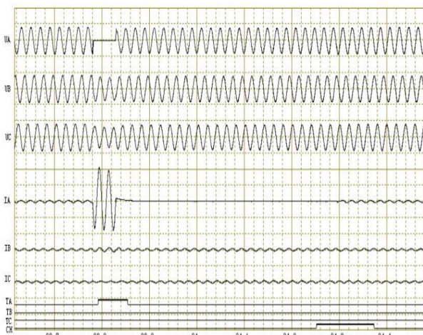
Figure 5 Single-phase transient metal ground fault inside zone
