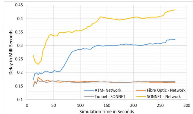
Fig. 7. ETE delay for GOOSE messages
