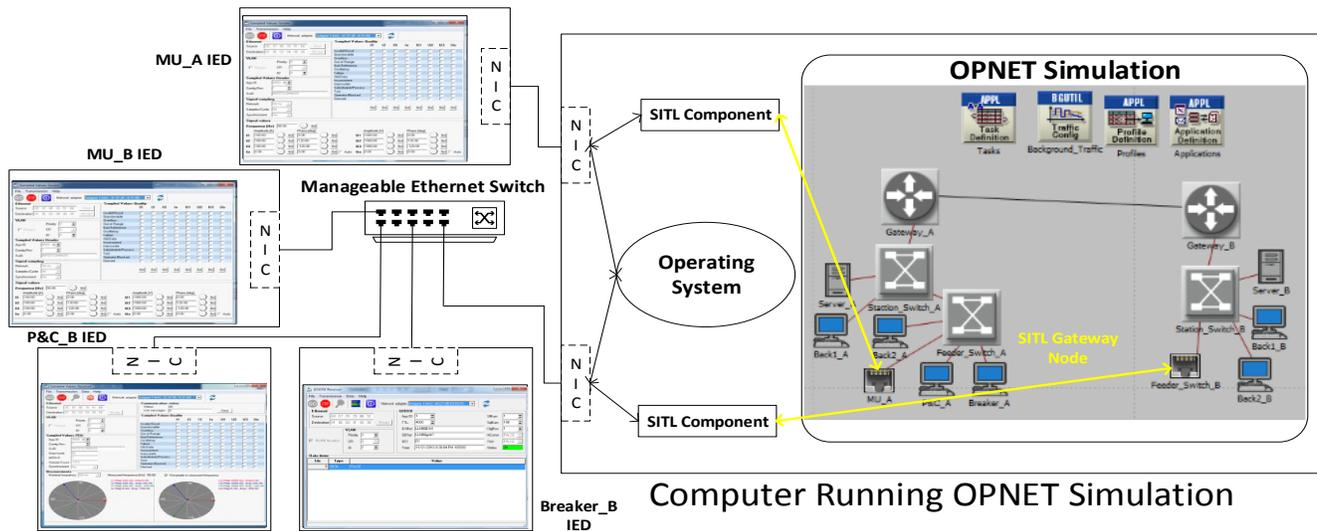
Fig. 8 SITL set up for differential protection between two substations
