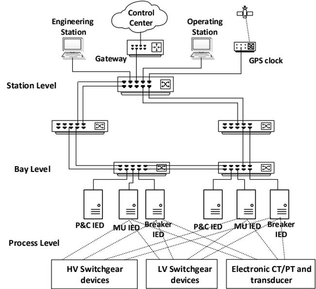
Fig. 3 IEC 61850 based substation communication architecture
