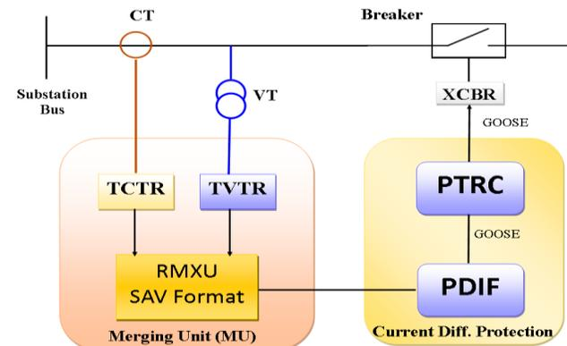
Fig. 2 Local Communication configuration of a substation
