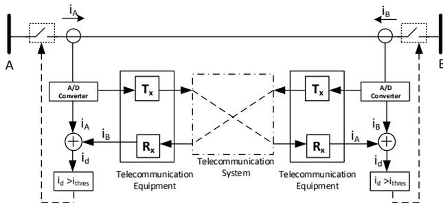
Fig. 1 Current differential protection scheme
