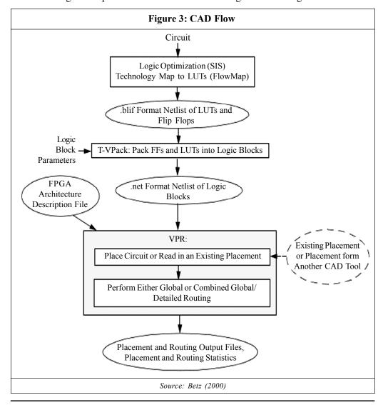
T-V pack is a packing program software which can be used with or without VPR. It takes a technology-mapped netlist consisting of Lookup Tables (LUTs) and Flip Flops (FFs) as input and then packs the LUTs and FFs together to form more coarse-grained logic blocks. The netlist as input is in .blif format and output is in the .net format. This output can be fed directly into VPR. T-V pack is invoked by typing:
