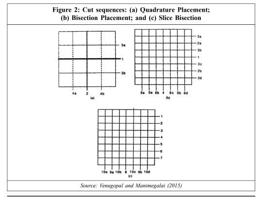
subregion contains only one slot. This process is most suitable when periphery has high interconnect density.
