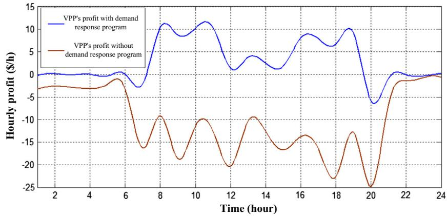
Fig. 11. The expected value of VPP's hourly profit for case 3.
