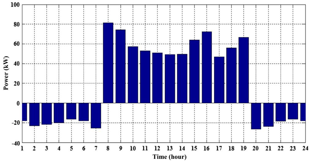
Fig. 9. The expected value of exchanged power between VPP and energy market for case 2.
