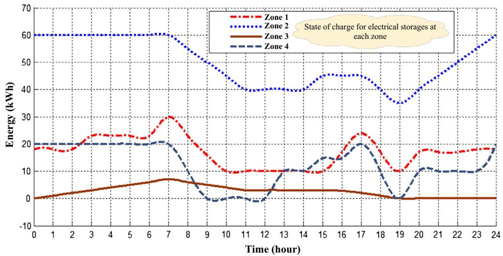
Fig. 10. The expected value of state of charge in electrical storages for case 2.
