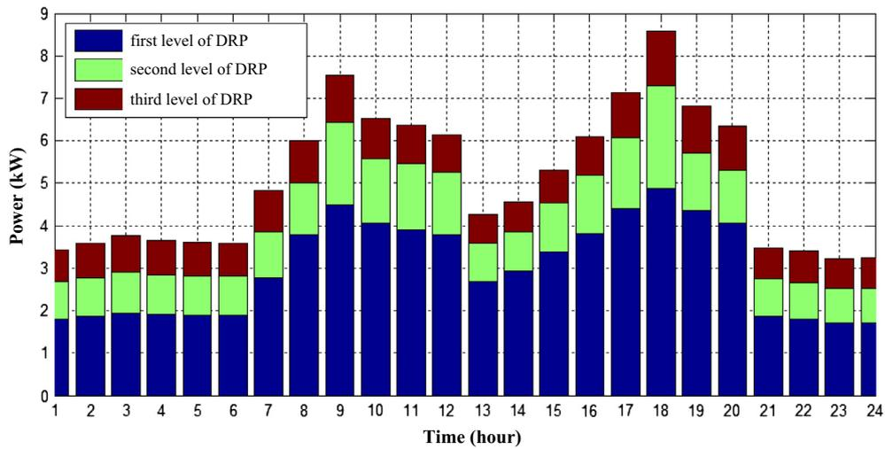
Fig. 12. The summation of curtailed power at each level of demand response program for all zones in case 3.
