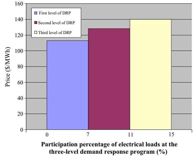
**Fig. 4.** The values pertaining to prices and allowable curtailed load of the three-level demand response program.
