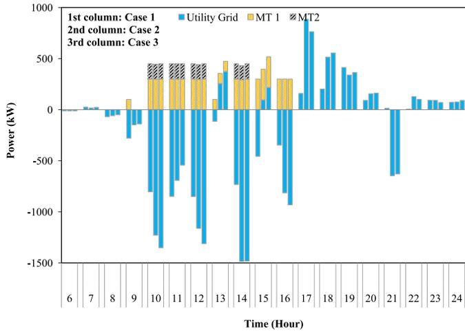
Fig. 7. Exchanged power between utility and IPL, and MTs outputs.
