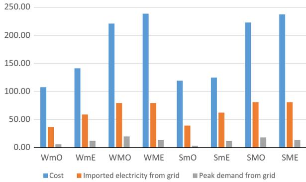
Fig. 8. Cost, imported electricity from grid, peak demand from grid comparison among different scenarios.
