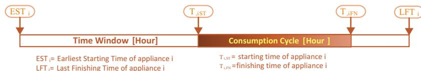
**Fig. 2.** ECAs' time window, consumption cycle, EST and LFT.
