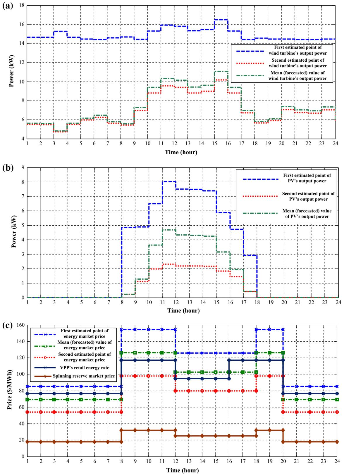
Fig. 5. Hourly forecasted, first estimated point and second estimated point for (a) output power of wind turbines, (b) output power of PVs, (c) energy market price in addition to contracted prices between VPP and end-consumers as well as spinning reserve market price and (d) VPP's electrical load power.
