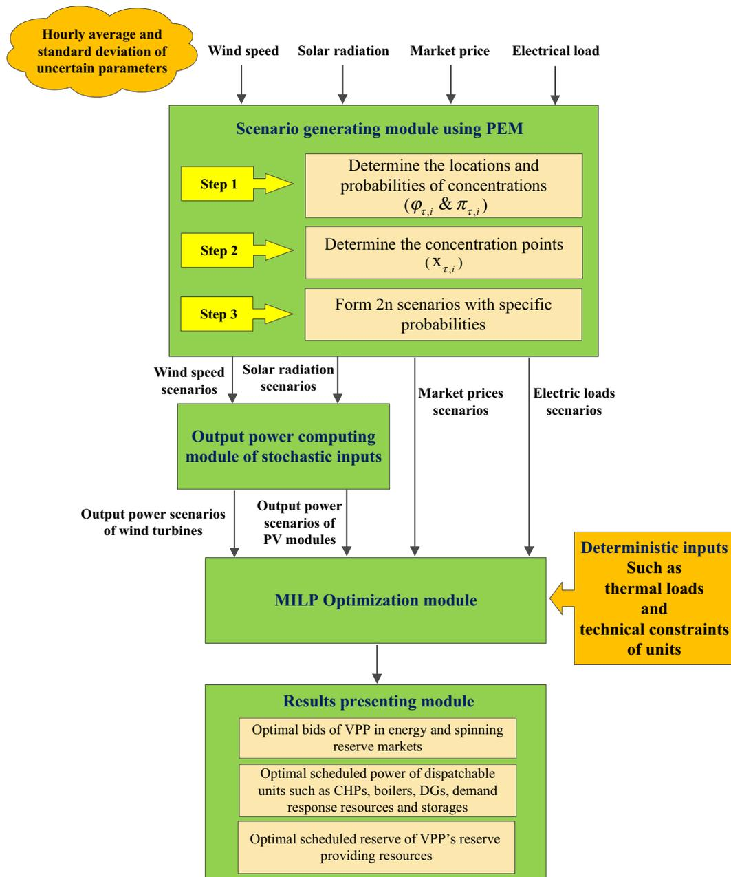
Fig. 3. The complete procedure of the proposed Probabilistic Mixed-Integer Linear Programming (PMILP) model using PEM.
