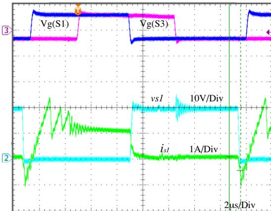
Fig. 14: Suppressed voltage oscillation in full-bridge stage in S.C. charge mode ( phase shift PWM control).
