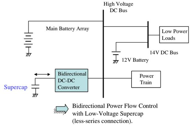
Fig. 1: Supercapacitor based energy storage system for automobiles.
