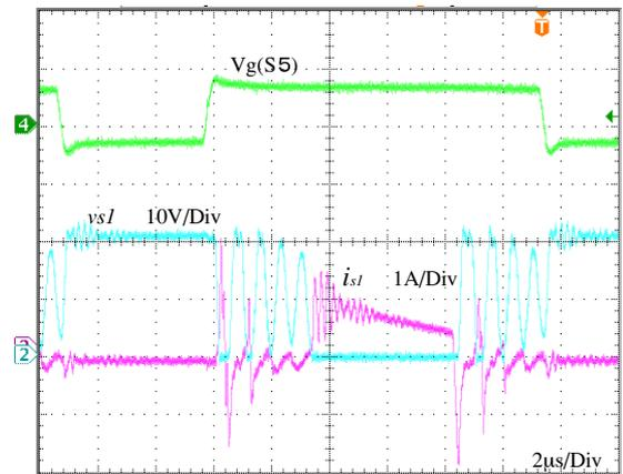
Fig. 13: Observed voltage oscillation in full-bridge stage in S.C. discharge mode (without S.R. in full-bridge side).
