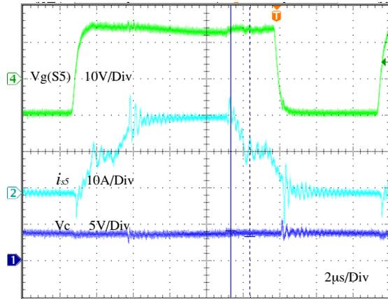
Fig. 10: Observed rectifying current in push-pull stage with Synchronous rectification (PWM control).
