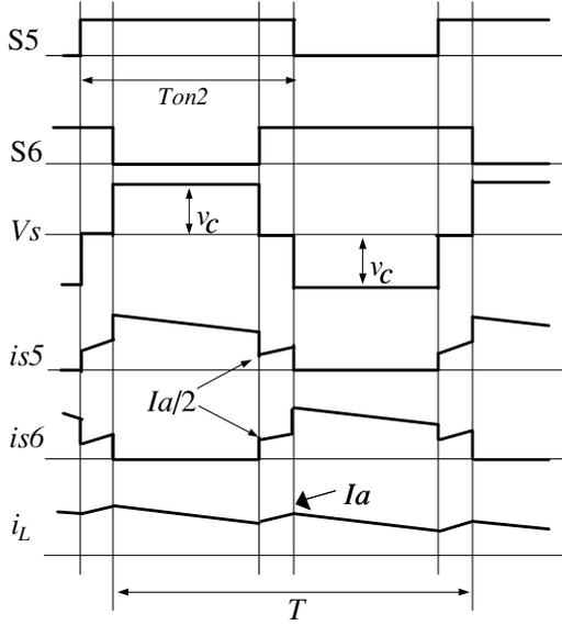
Fig. 6: S.C. discharge mode operation waveforms
