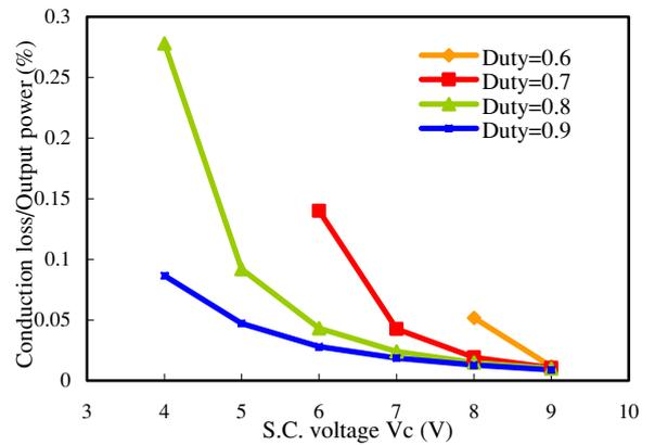
Fig. 16: Conduction losses in the rectifier device.
