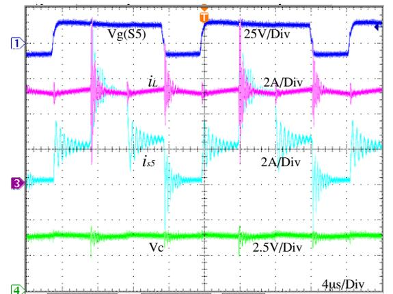
Fig. 8: Operating waveforms in S.C. discharge mode
