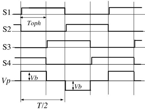
Fig. 4: S.C. charge mode operation waveforms (phase shift PWM control)
