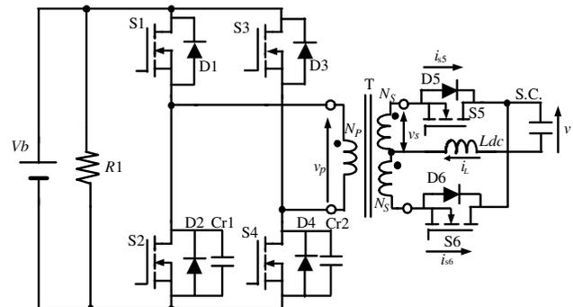
Fig. 2: Full-bridge/push-pull based bidirectional DC-DC converter
