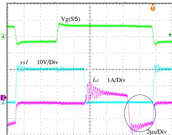
Fig. 15: Suppressed voltage oscillation in full-bridge stage in S.C. discharge mode ( with S.R. in full-bridge side).
