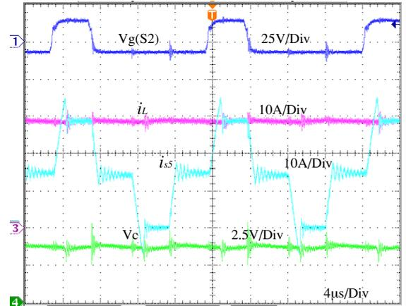
Fig. 7: Operating waveforms in S.C. charge mode without Synchronous rectification. (PWM control without lossless snubber capacitor)
