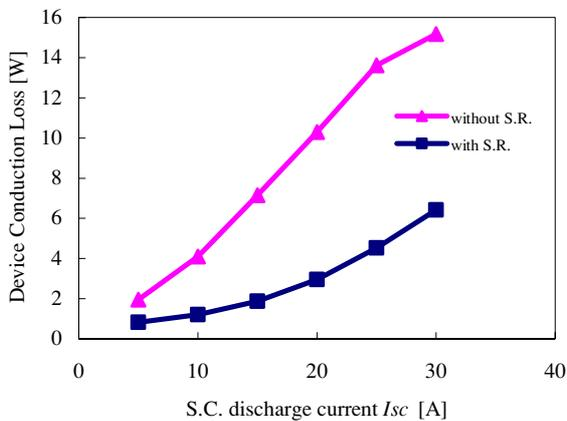
Fig. 11: Conduction losses reduction in the rectifier device.
