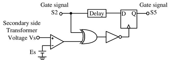
Fig. 5: Push-pull side synchronous rectification controller.
