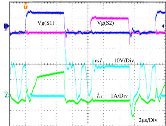
Fig. 12: Observed voltage oscillation in full-bridge stage in S.C. charge mode (PWM control).
