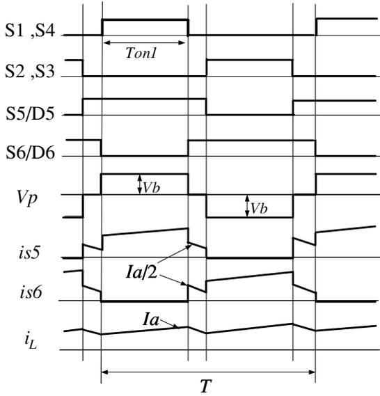
Fig. 3: S.C. charge mode operation waveforms (basically PWM control)
