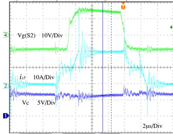
Fig. 9: Observed rectifying current in push-pull stage without Synchronous rectification (PWM control).
