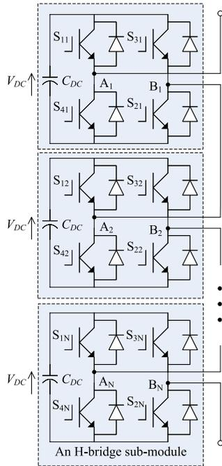
**Fig. 12. Cascaded H-bridge structure to generate staircase voltage waveforms.**
