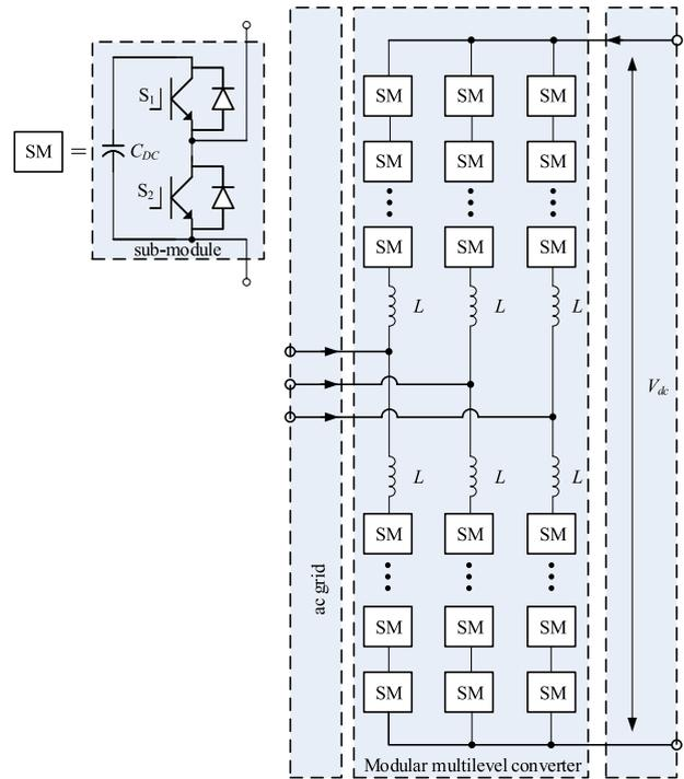
**Fig. 17. MMC for back-to-back configurations.**
