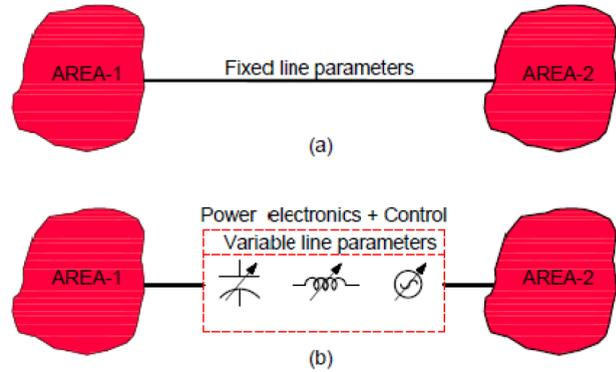
**Fig. 4. Role of power electronics in FACTS: (a) transmission network without FACTS and (b) transmission network with FACTS.**
