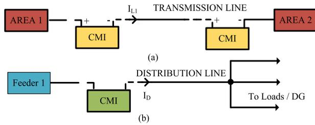
**Fig. 16. Series compensation using CMIs: (a) FACTS application and (b) RACDS application.**
