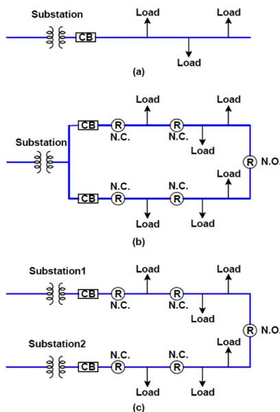
**Fig. 6. Different types of distribution network architecture: (a) radial, (b) ring, and (c) interconnected.**
