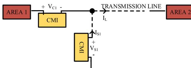
Fig. 19. Basic configuration of Transformer-less UPFC.
