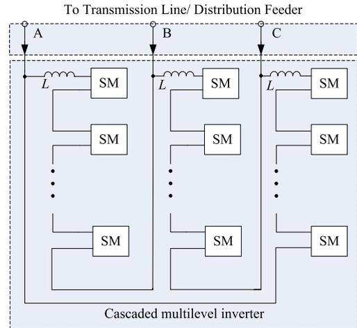
**Fig. 14. Delta connected CMI in shunt configuration.**
