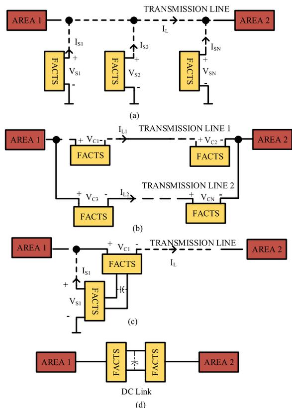
Fig. 8. Different configurations of FACTS for the smart-grid: (a) shunt, (b) series, (c) series-shunt, and (d) back-to-back.
