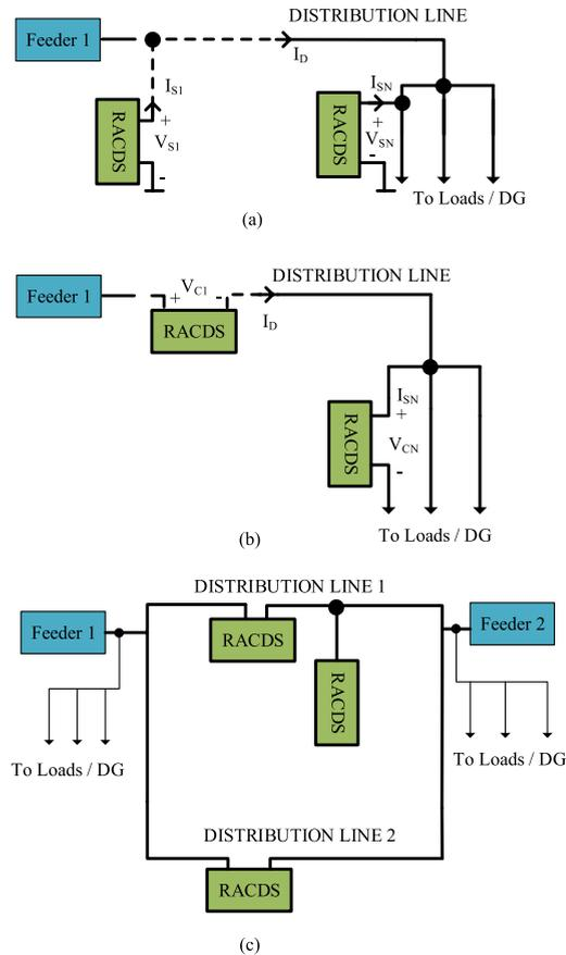
**Fig. 10. Different configurations of RACDS in the smart-grid: (a) shunt, (b) series and shunt, (c) series and series-shunt.**
