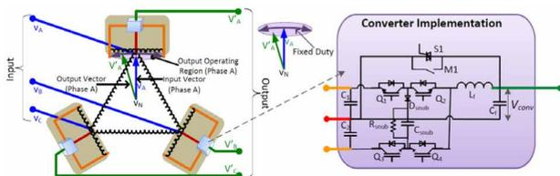
**Fig. 21. Structure of Compact-phase angle regulator [89].**
