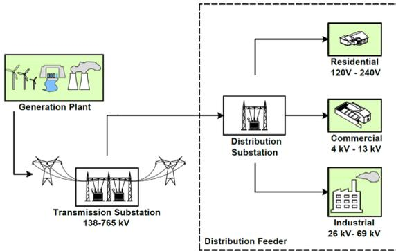
**Fig. 5. General layout of the power distribution network.**
