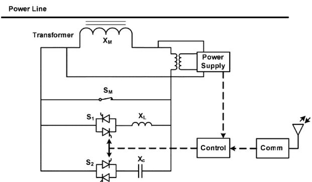
**Fig. 23. Floating Reactor implementation in distributed FACTS [90].**
