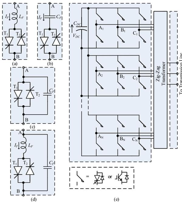
**Fig. 11. Basic building blocks of Traditional FACTS and RACDS devices: (a) TCR, (b) TSC, (c) TSSC, (d) TCSC, and (e) multi-pulse converter.**
