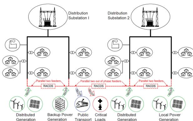
Fig. 9. Illustration of the distribution network in a smart grid.
