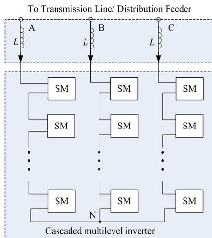
**Fig. 13. Wye connected cascaded multi-level inverter (CMI) in shunt configuration.**
