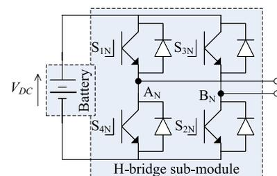
**Fig. 15. Battery integrated sub-module (SM) for CMI.**
