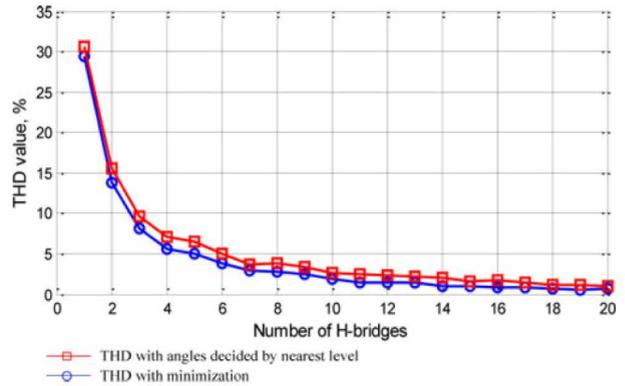
**Fig. 25. THD (%) versus number of modules for direct connection of cascaded H-bridge to power grid [61].**
