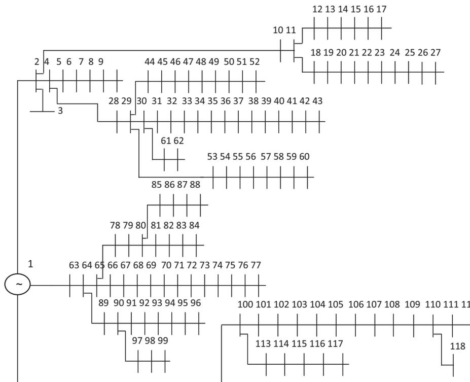
Fig. 8. The schematic diagram of the 118 bus system.
