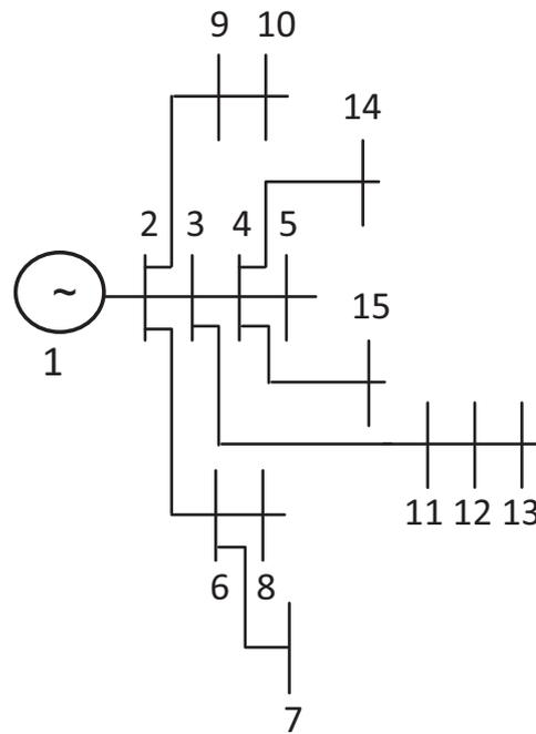
Fig. 2. The schematic diagram of the 15 bus system.
