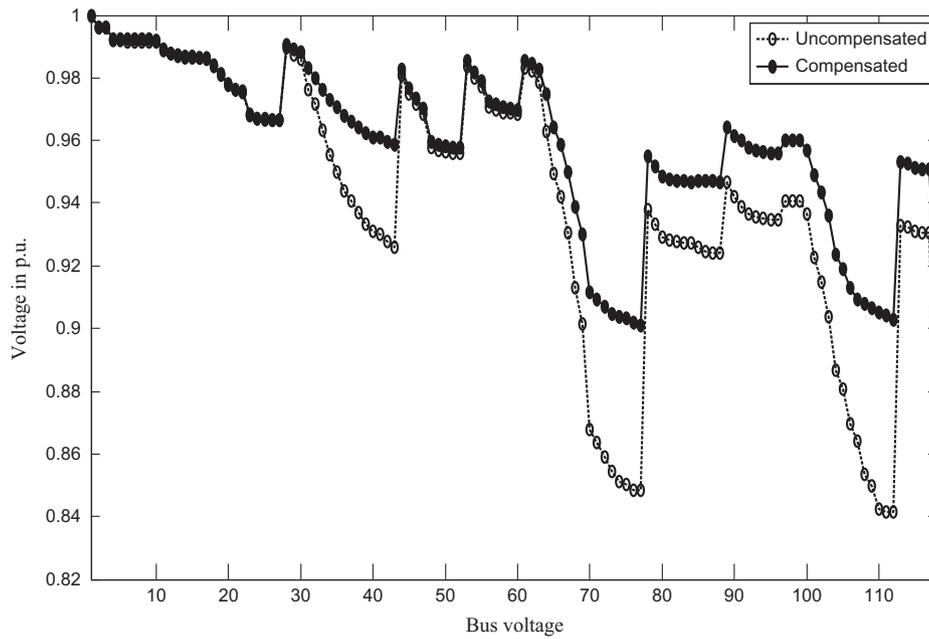
Fig. 10. Effect of compensation on system voltages.
