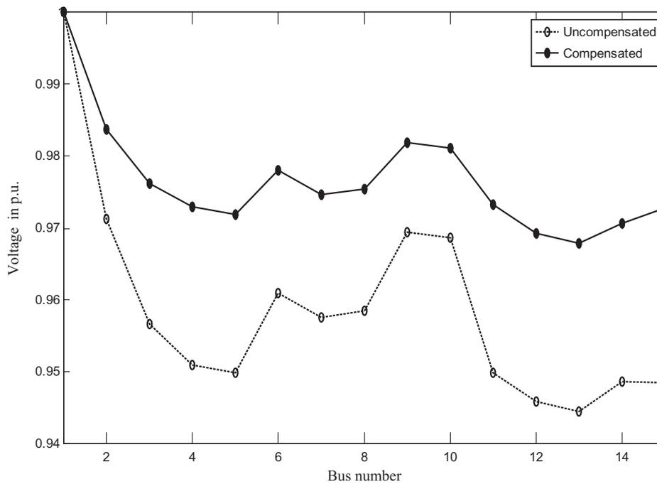
Fig. 4. Effect of compensation on system voltages.
