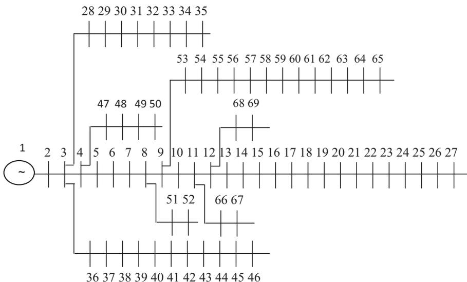
Fig. 5. The schematic diagram of the 69 bus system.
