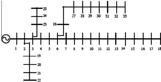
Fig. 5. Single line diagram of a 33-bus system.
