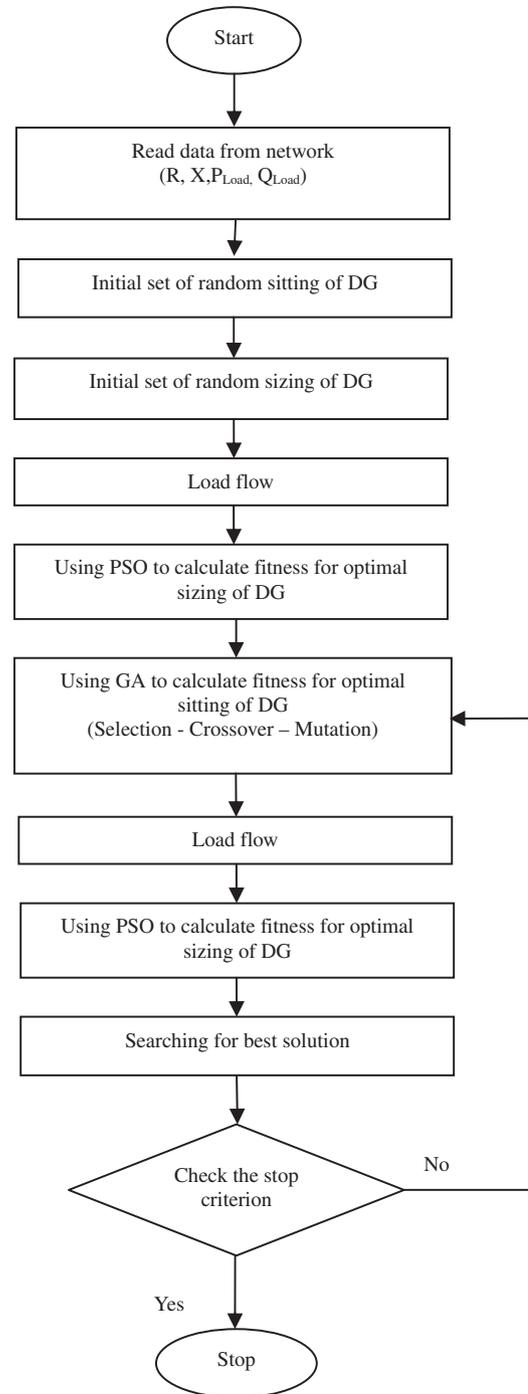
Fig. 4. The GA/PSO method for optimal sitting and sizing of DG.
