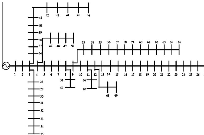
Fig. 8. Single line diagram of a 69-bus system.
