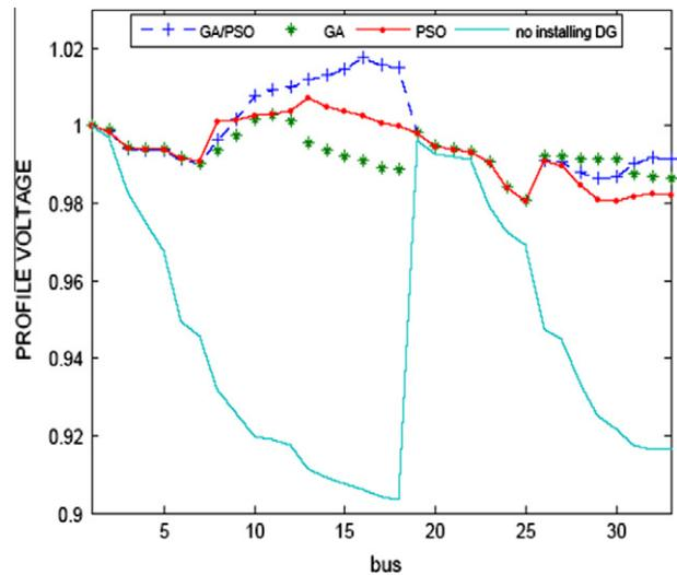
Fig. 6. Voltage levels of 33-bus radial distribution system.
