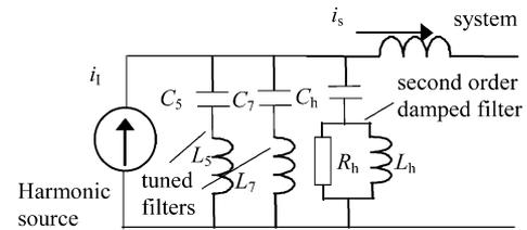
Fig. 2. Shunt passive filters for current harmonic source.
