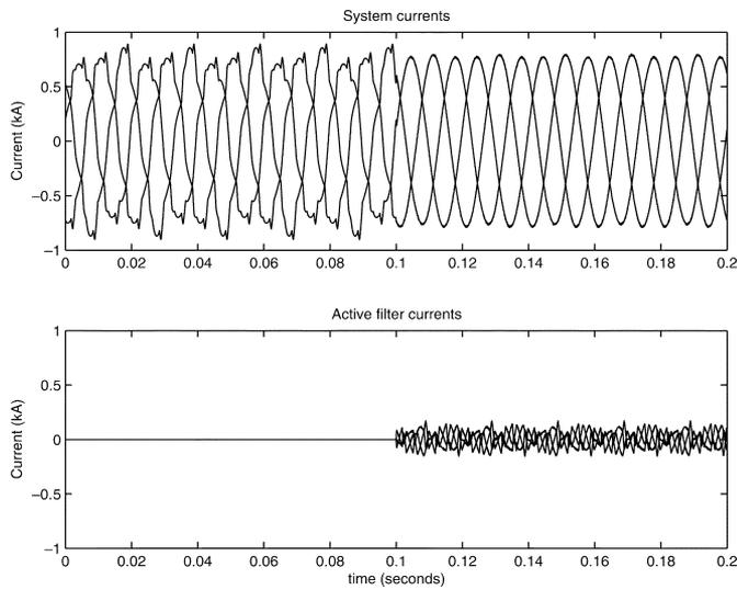
Fig. 17. System and active filter current waveforms (all DG units and loads in operation without passive filters).
