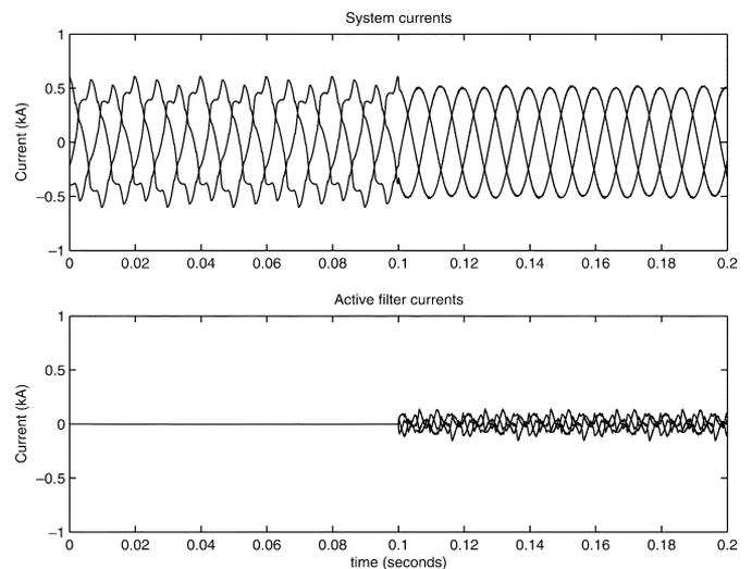
Fig. 15. System and active filter current waveforms (all DG units and loads with associated filters in operation).
