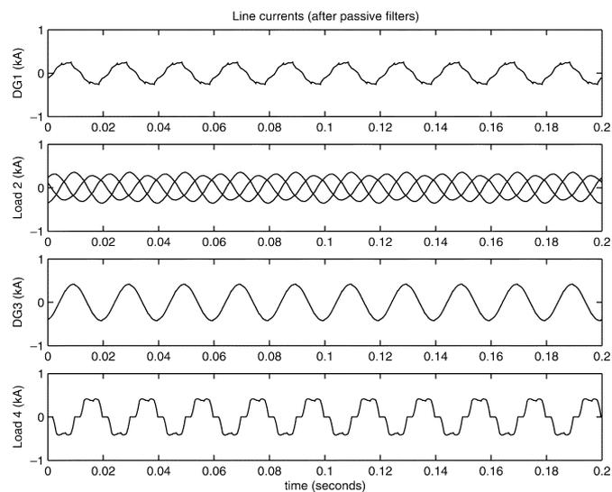
Fig. 14. Current waveforms in line branches (after passive filters).
