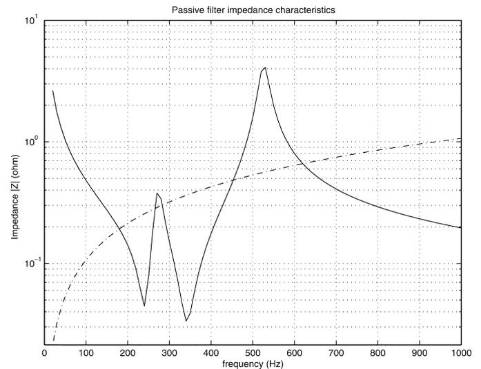
Fig. 3. Shunt passive filter characteristic.
