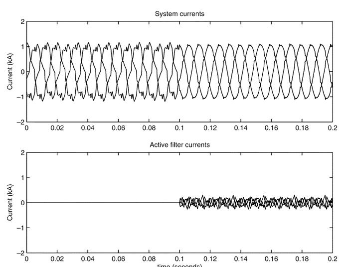
Fig. 20. System and active filter current waveforms (all four branch in operation without passive filters, short electrical distance).
