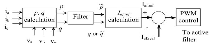
Fig. 5. Block diagram of control system for the active filter.
