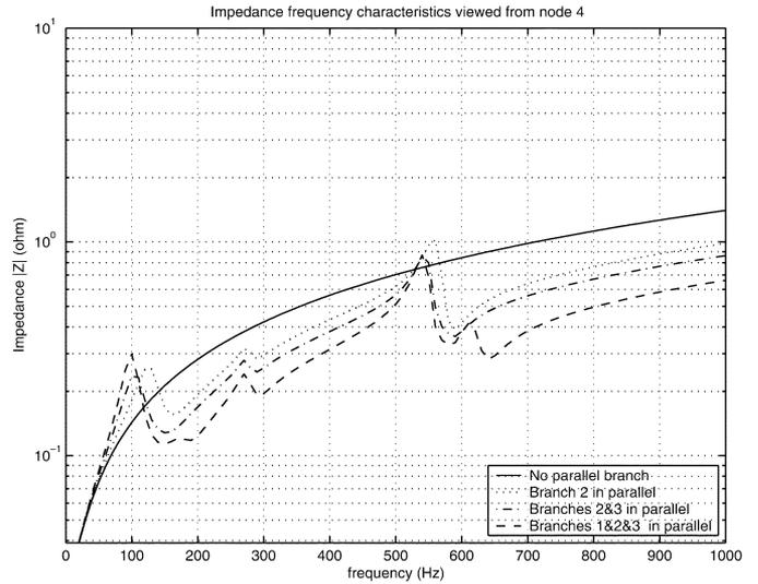
Fig. 12. Impedance characteristics viewed from node 4 in Fig. 6 (shorter electrical distance).
