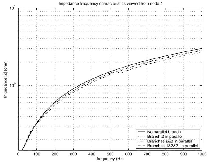
Fig. 11. Impedance characteristics viewed from node 4 in Fig. 6.
