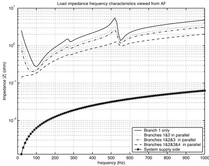
Fig. 9. Load impedance characteristics viewed from the active filter in Fig. 6.
