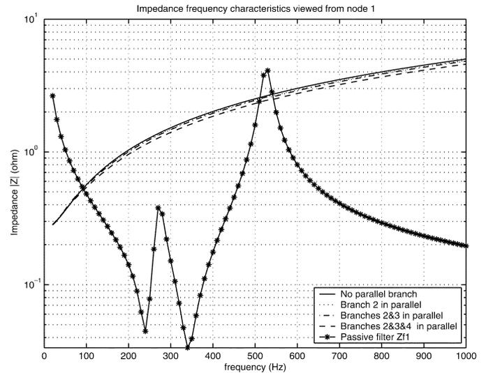
Fig. 7. Impedance characteristics viewed from node 1 in Fig. 6.
