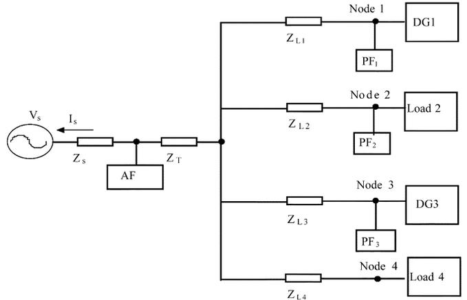
Fig. 6. Studied system configuration with dispersed generations and distorted load.
