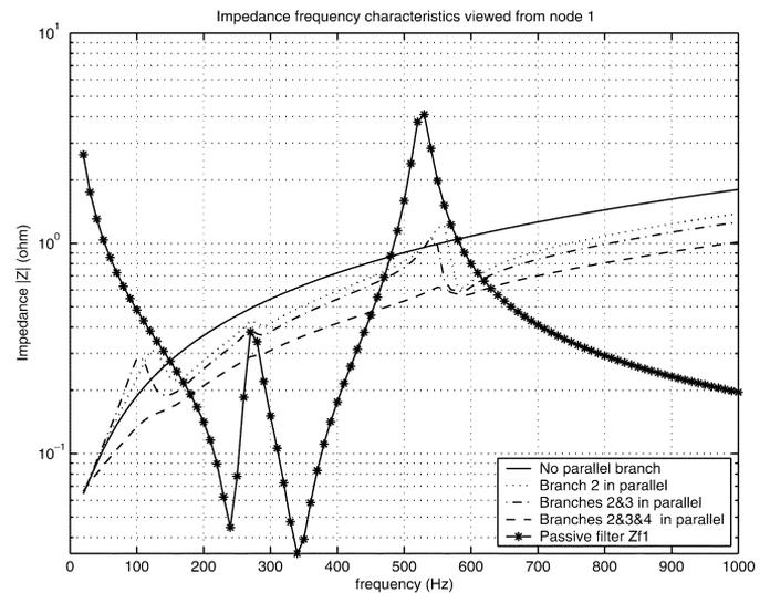
Fig. 8. Impedance characteristics viewed from node 1 in Fig. 6 (shorter electrical distance).
