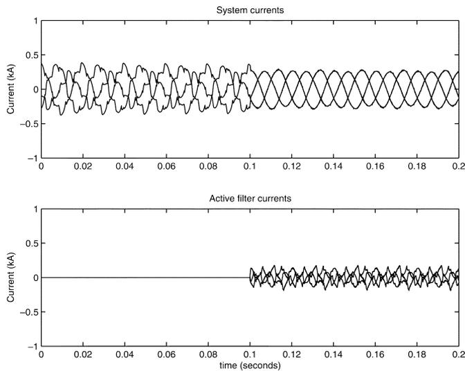
Fig. 18. System and active filter current waveforms (all four branch in operation, short electrical distance).
