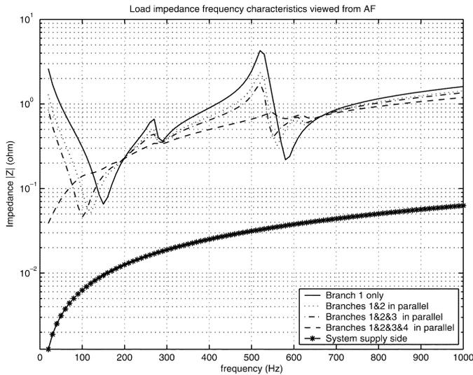
Fig. 10. Load impedance characteristics viewed from the active filter (shorter electrical distance) in Fig. 6.
