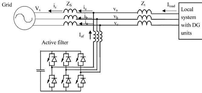
Fig. 4. An active filter for a current harmonic source.
