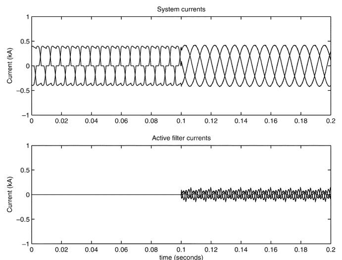
Fig. 16. System and active filter current waveforms (only load 4 in operation).
