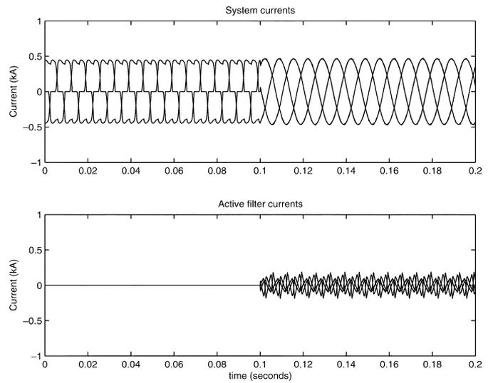
Fig. 19. System and active filter current waveforms (only load 4 in operation, short electrical distance).
