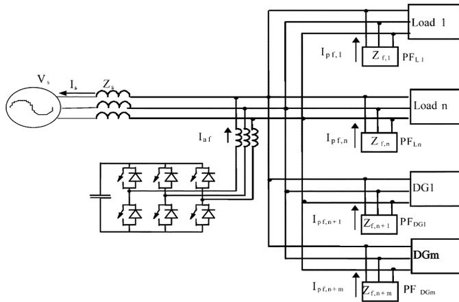
Fig. 1. Schematics of a parallel connected hybrid compensation arrangement in a system with dispersed generation (DG) units.
