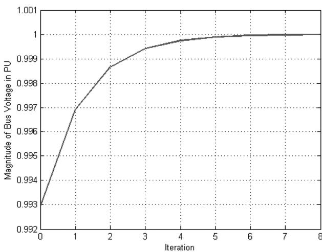
Fig. 6 Convergence curve of positive-sequence voltage of bus 740
