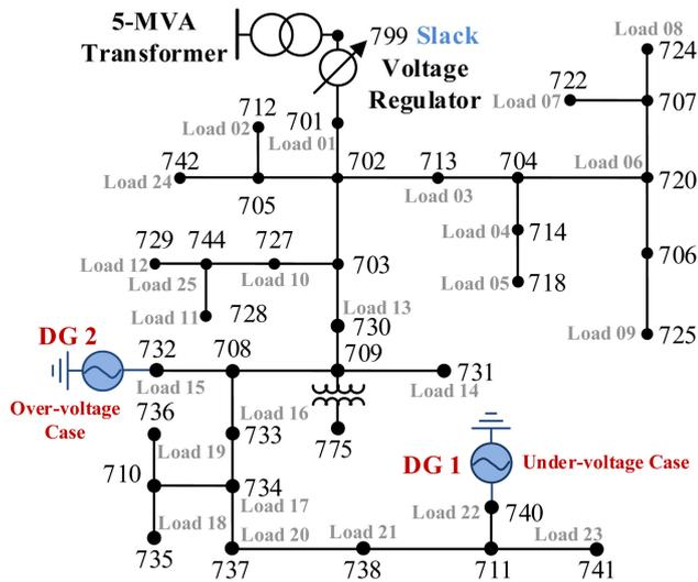
Fig. 5 IEEE 37-bus test feeder that hosts a DG system
