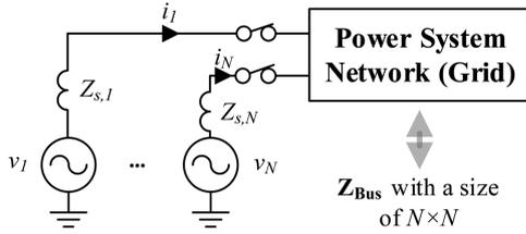
Fig. 2 Power system grid represented by the bus impedance matrix ( $Z_{Bus}$ )
