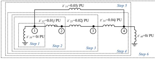
Fig. 3 Example of a power system network with four nodes
