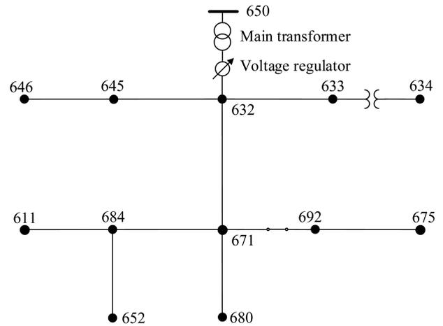
Fig. 11 IEEE 13-bus test feeder
