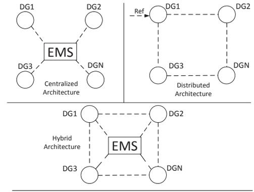
Figure 3. Communication Architectures for Reactive Power Control
