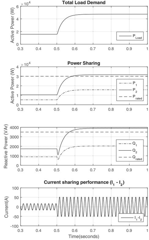
Figure 2. Transient response to a load change in a MG without power sharing control
