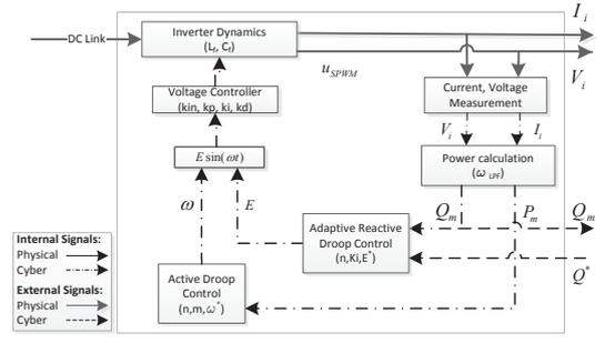
Figure 6. IDG CPES module (Adaptive Droop Control)
