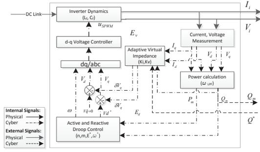
Figure 7. IDG CPES module. (Adaptive Virtual Impedance)
