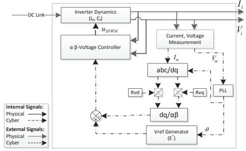
Figure 8. IDG CPES module. (SRF Virtual Impedance Loop)
