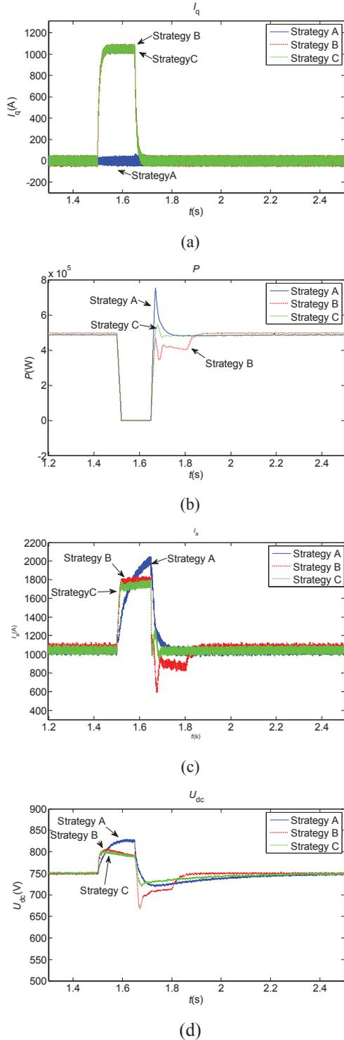
**Fig.4:** Simulation results with the zero voltage fault (a) Reactive current, (b) Active power, (c) Magnitude of the grid side current (d) DC-link voltage.
