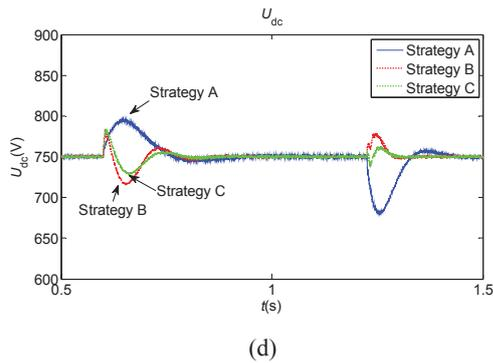
**Fig.5:** Simulation results with the 70% voltage dip (a) Reactive current, (b) Active power, (c) Magnitude of the grid side current (d) DC-link voltage.
