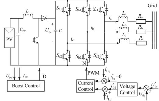
**Fig. 2:** Schematic diagram of the PV system
