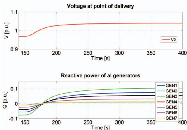
Figure 10. Generators reactive powers and voltage response in network C with decoupling matrix.
