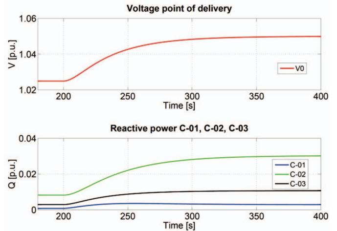
Figure 8. Voltage and reactive power response for a step in reference voltage with the decoupling matrix: network B .
