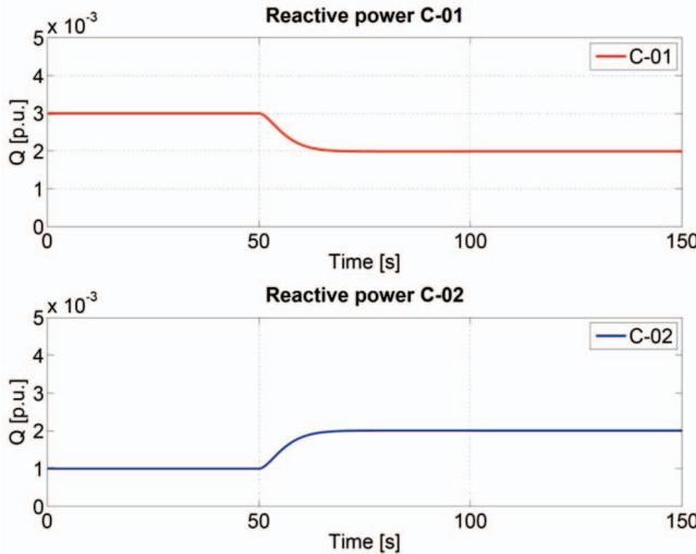
Figure 6. Reactive power response with dynamic decoupling.
