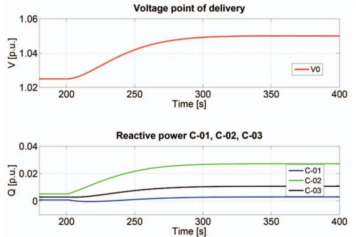
Figure 7. Voltage and reactive power response for a step in reference voltage without the decoupling matrix: network B
