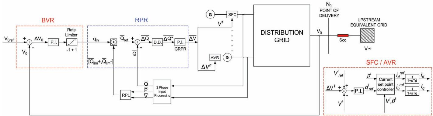
Figure 1. Synoptic schema of the secondary voltage control.
