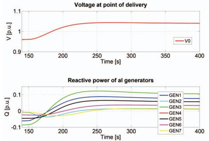
Figure 9. Generators reactive powers and voltage response in network C without decoupling matrix
