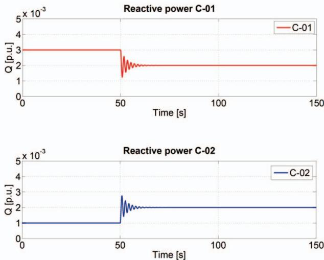
Figure 5. Reactive power response without dynamic decoupling.
