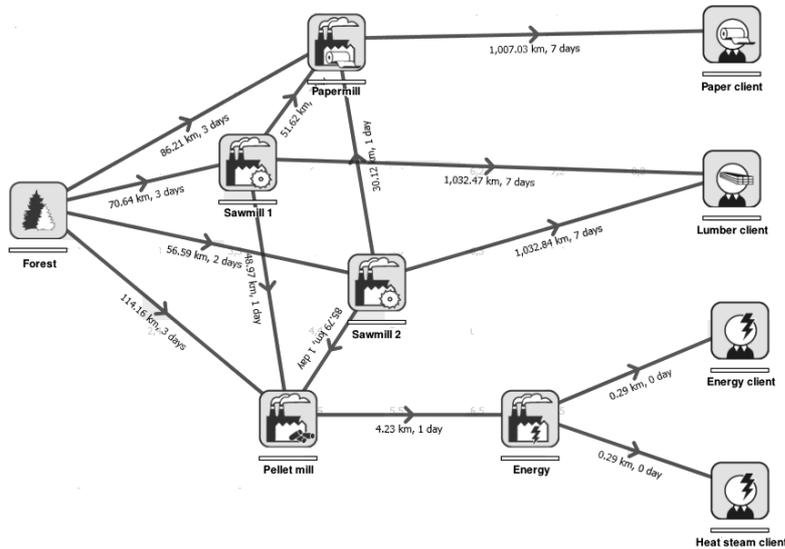
Figure 2: Network representation of the value chain optimization problem. The distances between the production units and the transportation time are indicated.
