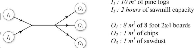
Figure 3: A typical transformation process in the value chain optimization model.
