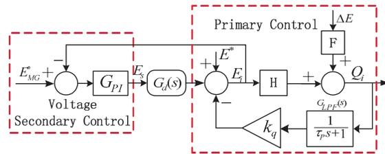
Fig.6 Structure of distributed secondary control with time delay
