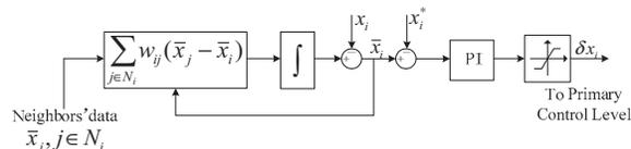
Fig.3 State observer and compensation value
