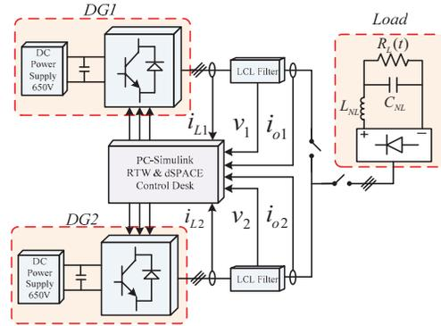
Fig.4 Simulation setup of an islanded MG with two DG units
