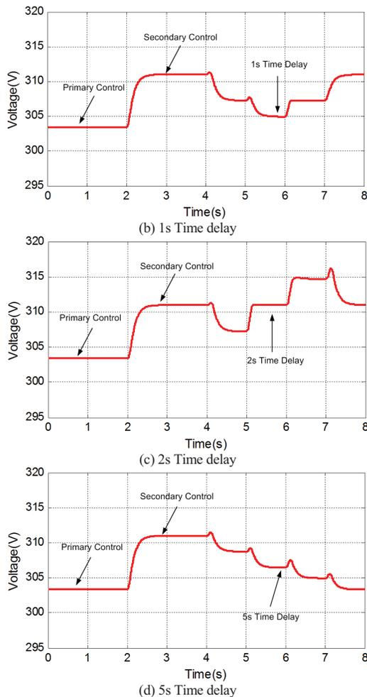
Fig.7 Dynamic performance evaluation of DSC with time delay
