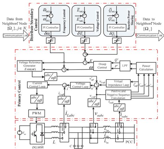
Fig.2 Scheme of distributed hierarchical control for a DG unit
