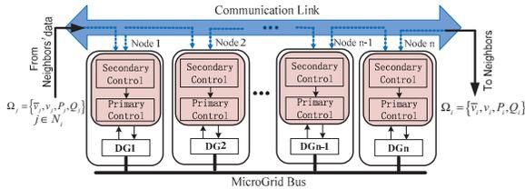
Fig.1 Proposed hierarchical control architecture for islanded MGs
