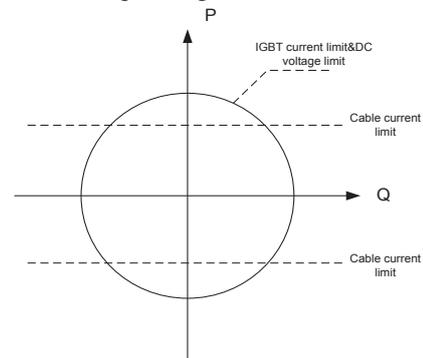
Figure 10 Typical PQ curve of VSC HVDC system
