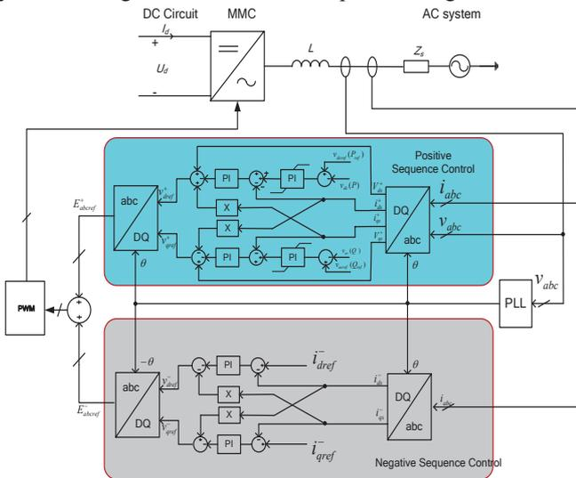
Figure 3: Control system for MMC converter
