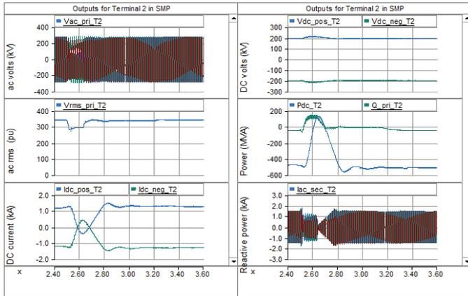
Figure 15: AC quantities at terminal 2 for LG fault
