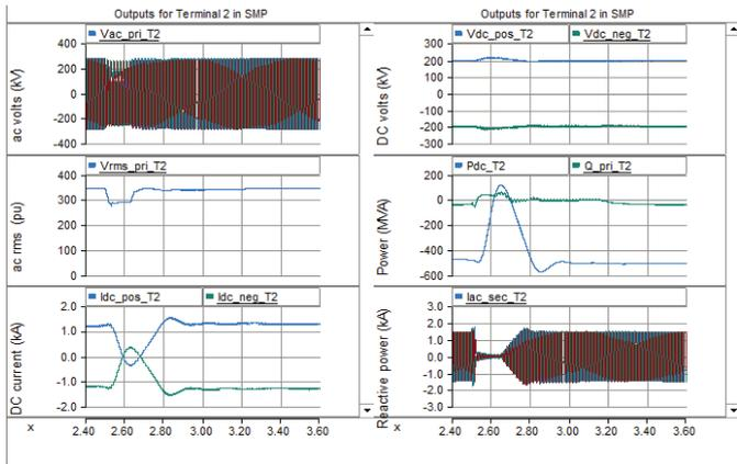
Figure 7: AC and DC quantities at terminal 2 in LG case
