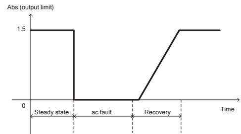
Figure 5: The change of the PI controller limit
