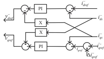
Figure 14 Negative sequence control with reactive current compensation
