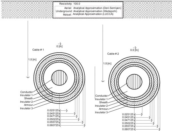
Figure 2: DC cable parameters in EMT model
