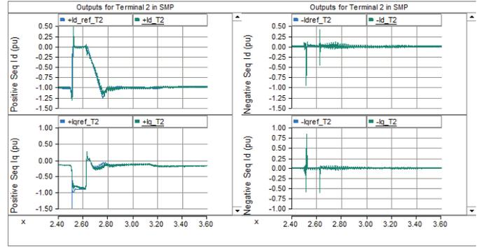
Figure 13: Id and Iq currents for 3LG fault
