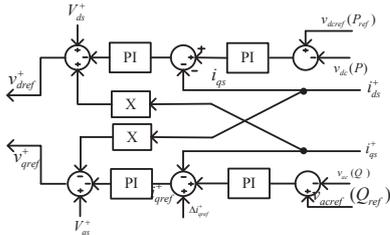
Figure 11 Positive sequence control with reactive current compensation
