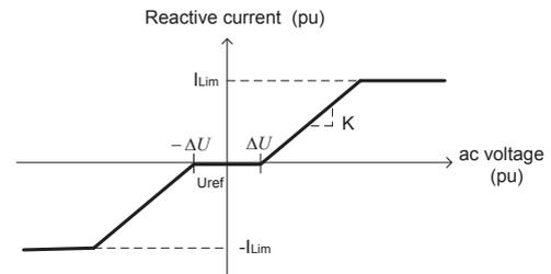
Figure 9: Reactive current compensation vs voltage deviation
