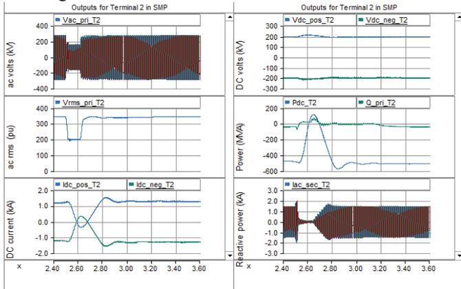
Figure 6: AC and DC quantities at terminal 2 in 3LG case
