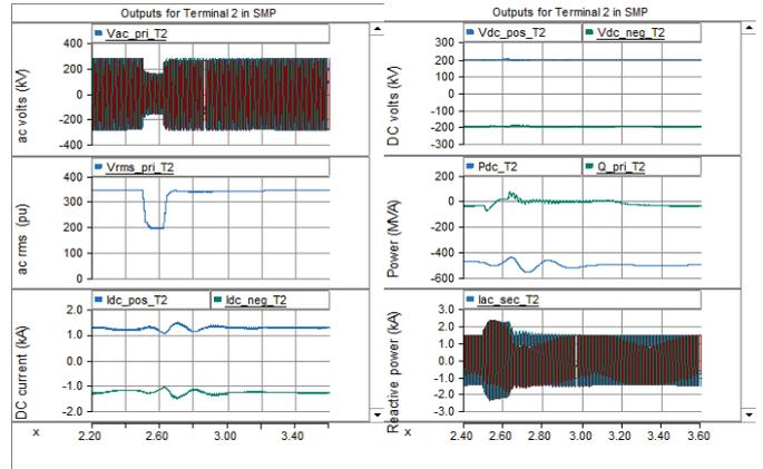
Figure 4: overcurrent in the converter during 3LG fault
