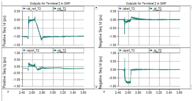
Figure 16: Id and Iq currents for LG fault
