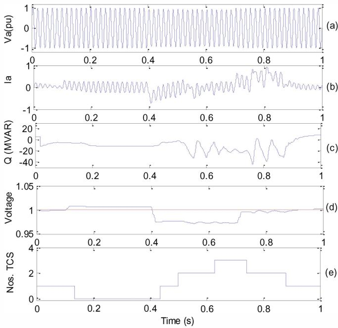
Fig. 4. Variations in amplitude of phase-A (a) voltage (b) current (c) reactive power (d) measured voltage and reference voltage (e) number of TCS utilized.
