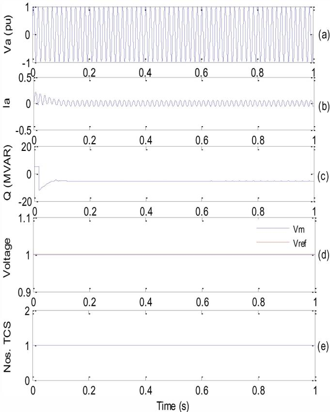
Fig. 2. Healthy condition (a) voltage (b) current (c) reactive power (d) measured voltage and reference voltage (e) number of TCS utilized.
