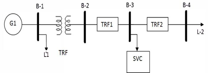
Fig. 1. Single line diagram of the proposed test system.
