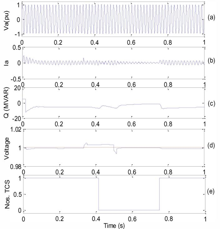
Fig. 6. Switching of the load L1 (a) voltage (b) current (c) reactive power (d) measured voltage and reference voltage (e) number of TCS utilized.
