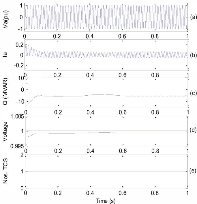
Fig. 5. Switching of the load L2 (a) voltage (b) current (c) reactive power (d) measured voltage and reference voltage (e) number of TCS utilized.
